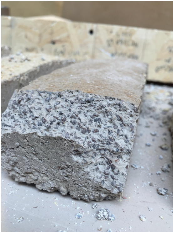
Figure 184. The dry sample 4. The edges were crumbled without excessive force. Photo: Andi Dani
