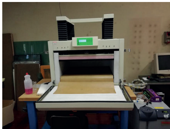
Figure 82. The Lasercomp FOX600 where the hot plate tests are performed.
