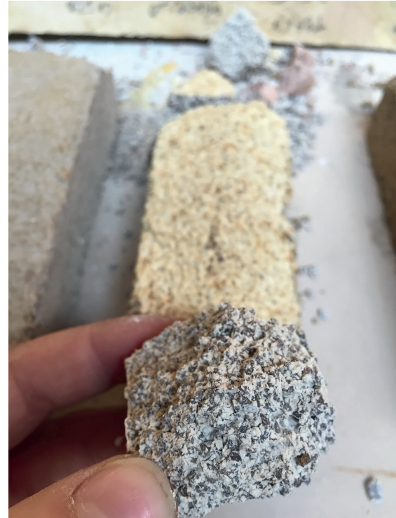
Figure 192, 193 (left) and 194 (above). Dried sample 6 showing a very fragile behaviour and olive stains, mostly on the top surface.
