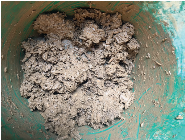
Figure 112. Earth from unfired bricks and hemp shiv wet mix.
