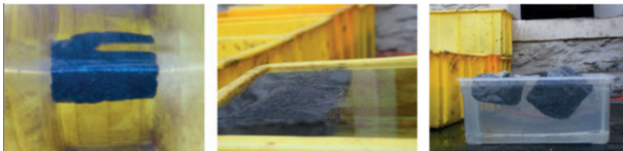
Figure 213, 2014 and 2015. Biochar bricks floating on water.
