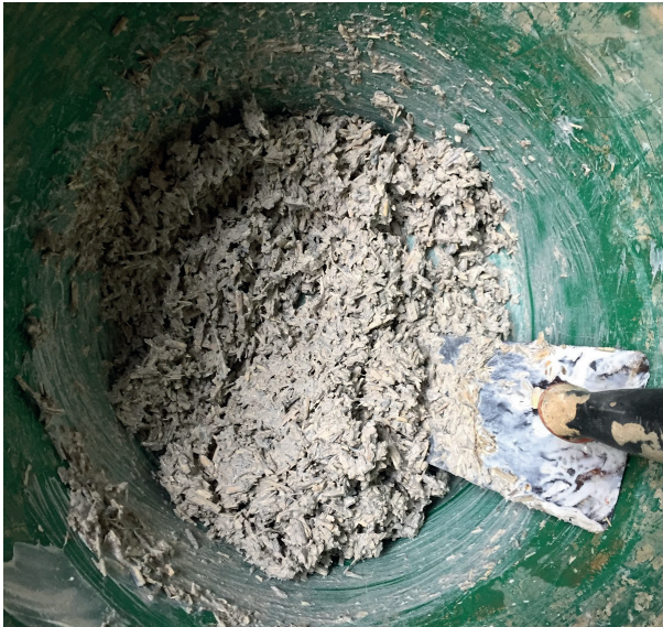
Figure 125. Hemp shiv, lime putty and NHL 5 after being mixed with a trowel.
