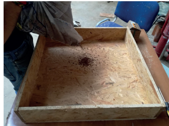
Figure 161 (above), 162, 163, 164 and 165 (next page). The preparation of the crushed olive pits sample which was sent to the laboratory of the Department of Energy of the Politecnico di Torino for the Hot Guarded Test.
