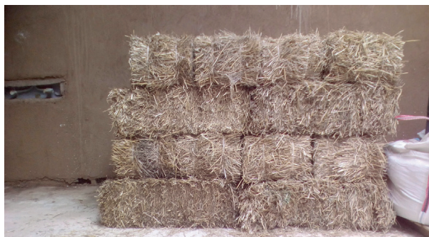
Figure 83. The rectangular rice straw bales used for the lime straw insulation inside the Red Room.
