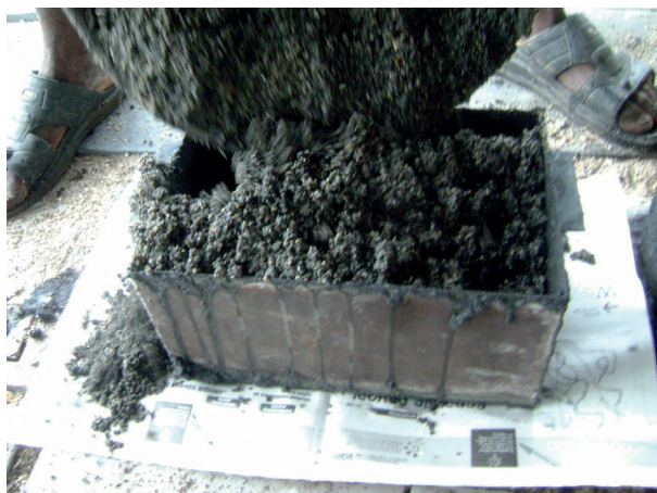
Figure 218 and 219. After wet biochar is mixed with sand, Portland cement is subsequently added (above). Once the ingredients are mixed and a homogenous composite is obtained, they are inserted in a form which gives the biochar brick its shape (below). Source: http://e-biocharbricks.blogspot.com/
