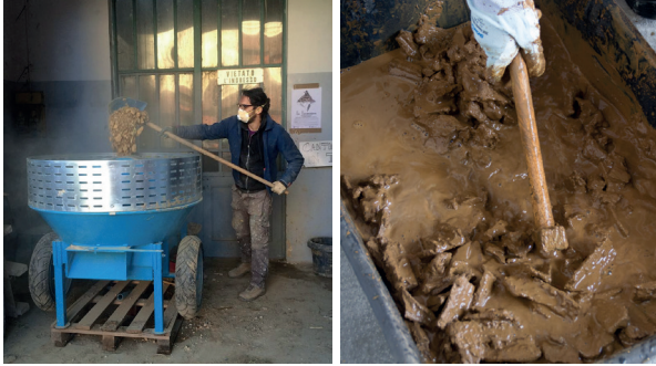
Figure 64 and 65. On the left, the process of crushing the unfired bricks, passing them through a sand mix mill. On the right the process of preparing the clay slip from the crushed bricks. Photos: Arthur Bohn
