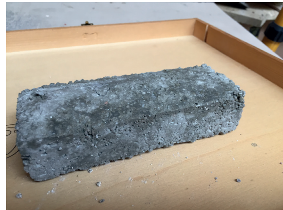
Figure 198. Sample 7 once dried. Oil stains can be noticed on the surface.
