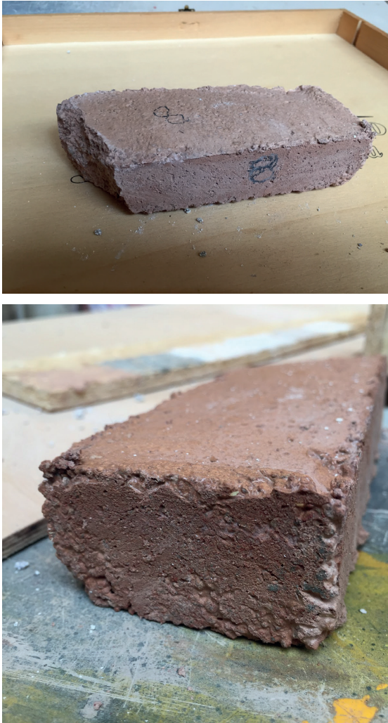
Figure 203 and 204. Pictures of dried sample 8. No noticeable oil stains are shown Photo: Andi Dani
