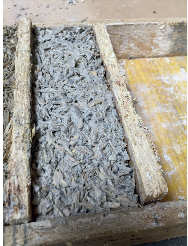
Figure 126. Hemp shiv, lime putty and NHL 5 mix cast inside the woodform once it had reached a homogenous state.
