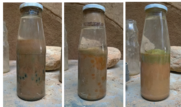
Figure 53. The sedimentation test results. The first bottle contains the earth from the crushed bricks, the second the dark subsoil earth and the third one the yellow subsoil earth.
