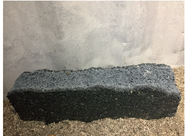
Figure 226. The sample produced by mixing hemp shiv, NHL 5 and charcoal. Photo: Andi Dani
