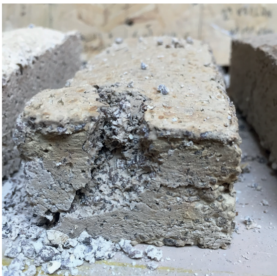
Figure 187 and 188. The dry sample was easily broken and crumbled. The oil is seen on the surface where it has created brownish stains.
