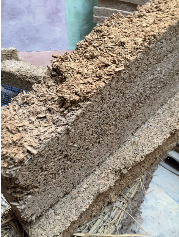
Figure 114. Earth from unfired bricks and hemp shiv 40x50x10 cm sample.
