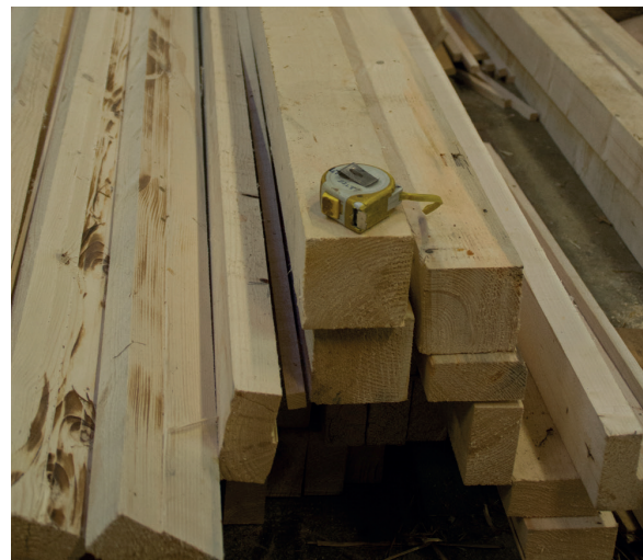
Figure 54. The wooden joists used to build the studs. Initially it was thought to employ 10x10 cm section elements, but this was found to be excessive. The joists were therefore cut in half, reducing them to a 5x10 cm section.
