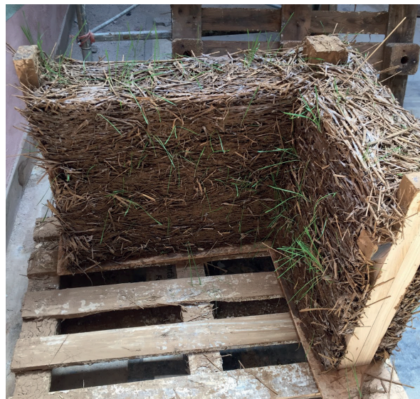
Figure 69. Light earth insulation life size model that simulates an angle when this material is used as infill material. The mixing process is the same as when light earth mix is used to insulate existing walls.
