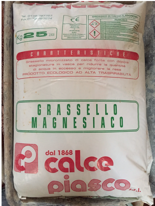
Figure 89. The lime putty used for the preparation of the lime straw mixture. It is a 25 kg sack of micronised slaked lime, double aged in tanks in order to reduce the excessive water. It was obtained from the Calce Piasco company. It is specified that this lime putty derives from magnesium limestone.
