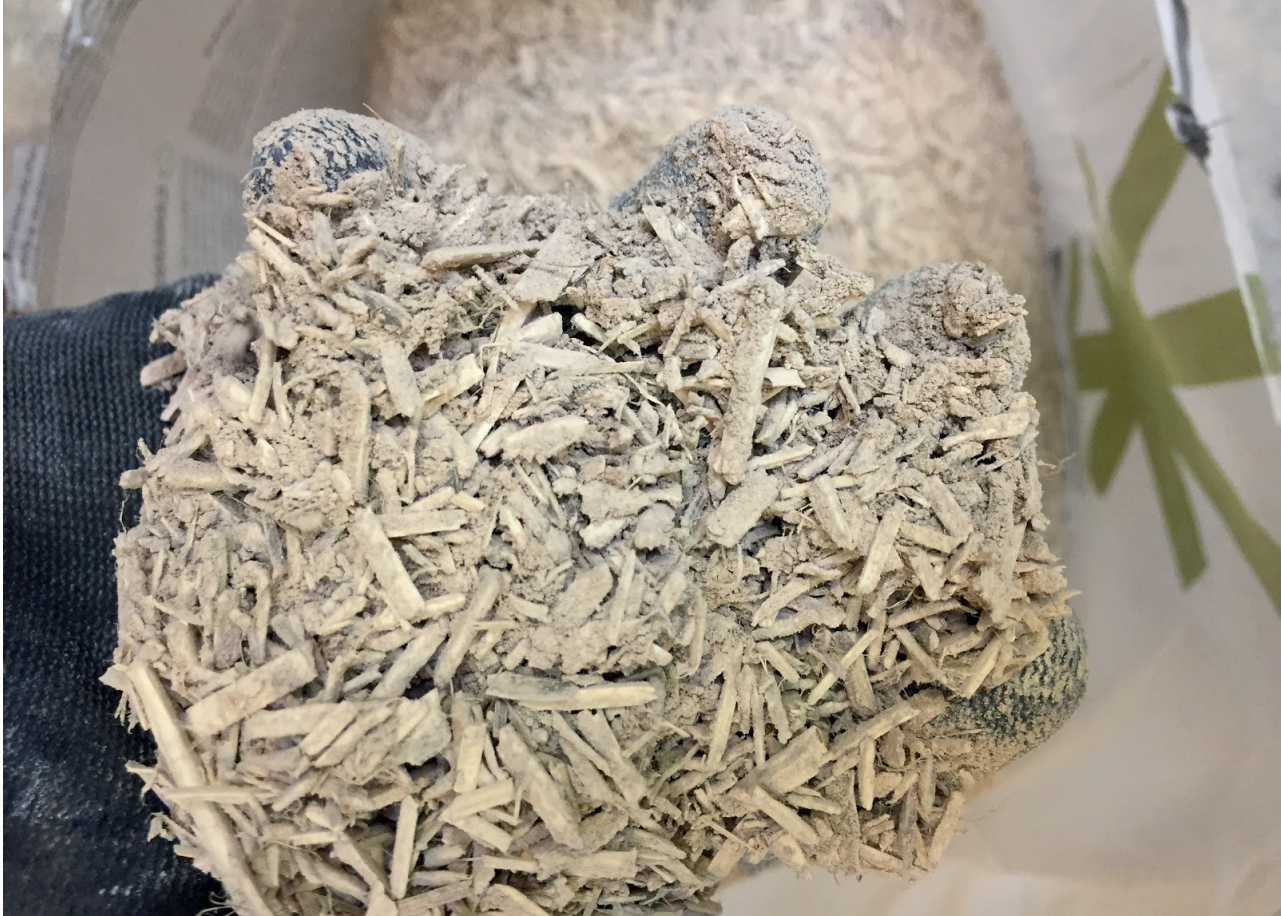
Figure 108. The hemp shiv in the premixed product obtained from Edilcanapa. This shiv is already mixed with a specific hempcrete binder.
