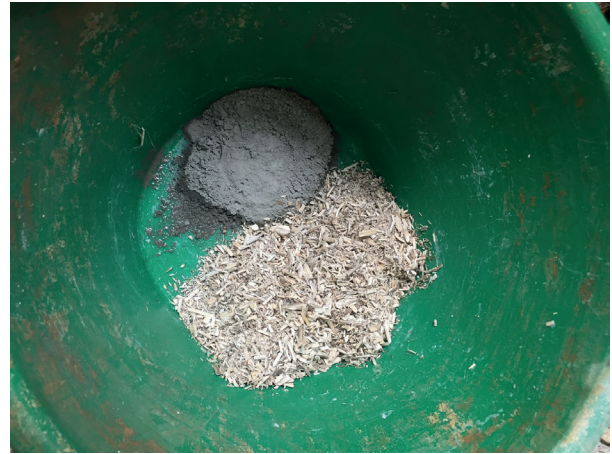
Figure 134. Portland cement and hemp shiv inside a clean bucket before being mixed.
