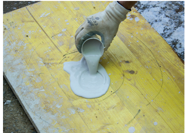
Figure 92. The lime slip density test taken over a smooth wooden board where circles with 20 and 30 cm diameters were previously drawn.
