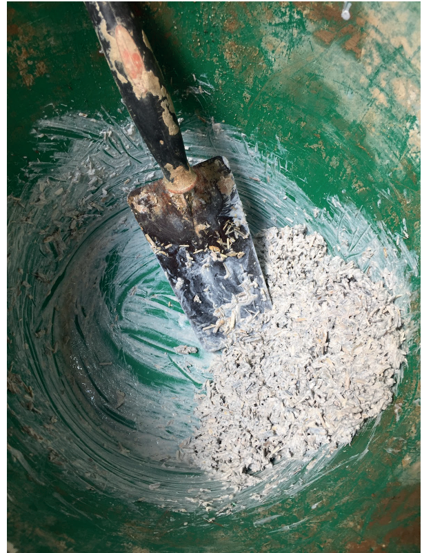
Figure 119. The lime putty-hemp shiv wet mix
