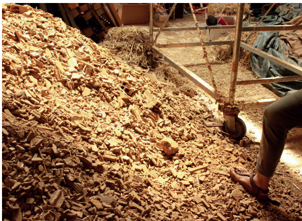
Figure 52. Crushed bricks used as a binder for the straw clay insulation
