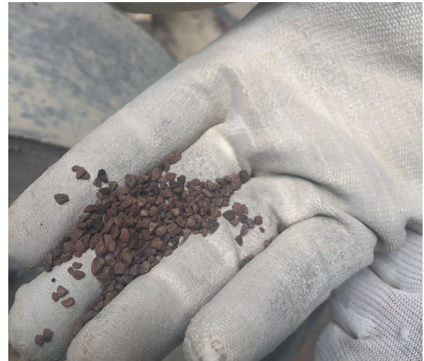
Figure 159 and 160. Crushed olive pits (human hand as reference).
