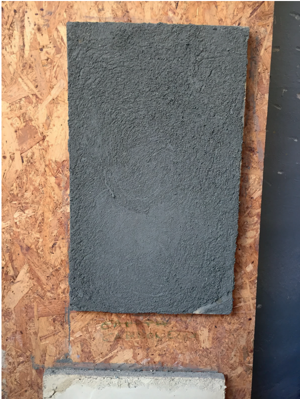
Figure 210. One of the samples of charcoal plaster where the char consisted in 40% of the mix. Photo: Andi Dani
