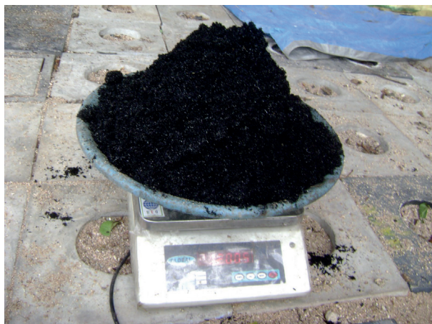
Figure 216. For the production of biochar bricks, the biochar material is first saturated, being the quickest ingredient to absorb water. The wet biochar is then mixed with sand, and the last ingredient to be added is the cement.
