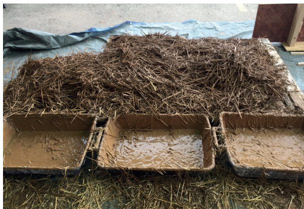
Figure 68. Straw dipping in clay slip. If the straw stems are soaked, they can get more clay binder attached to them and subsequently, they can create a denser composite compared to when clay slip is poured over the straw. This would increase the mechanical properties of the panels, but it would reduce its thermal performance as an insulation material. Photo: Andi Dani
