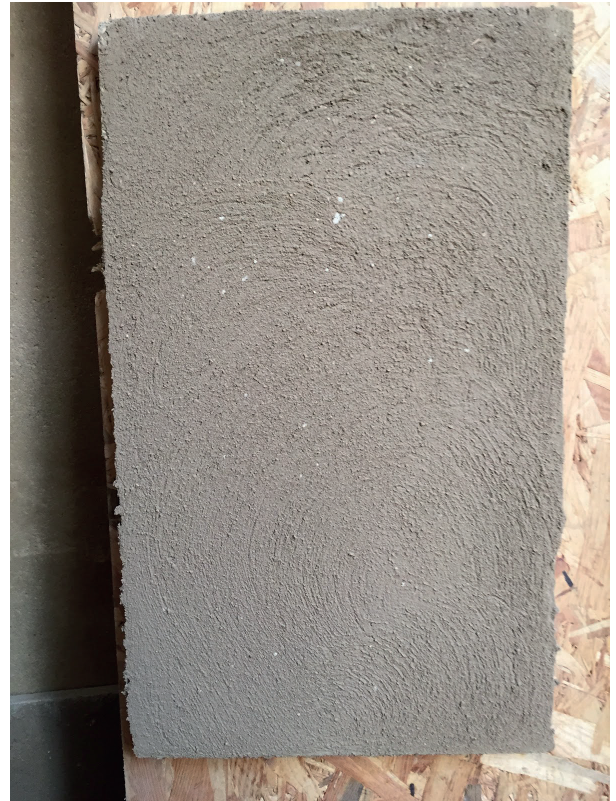
Figure 211. The charcoal plaster sample where the char consisted in 20% of the mixtures weight. The smaller the quantity of char (biochar) added to the mix, the lighter the plaster colour and the slower the drying time. Photo: Andi Dani
