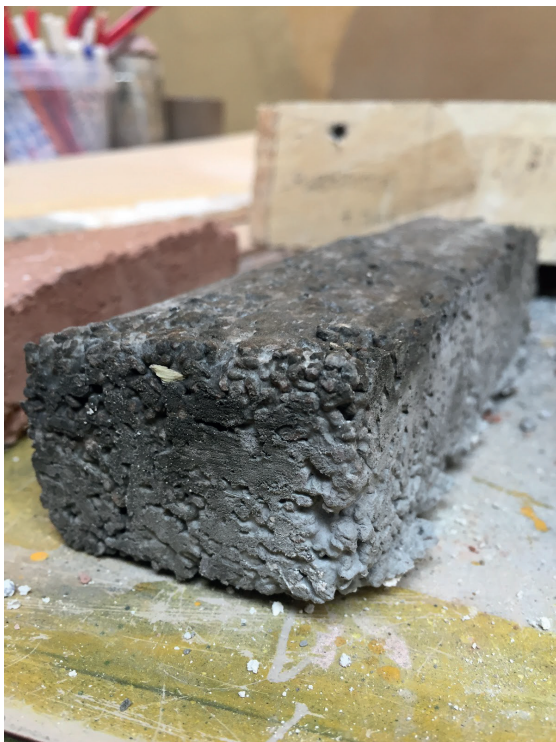
Figure 199. Oil manifestation on the top surface of dried sample no. 7.
