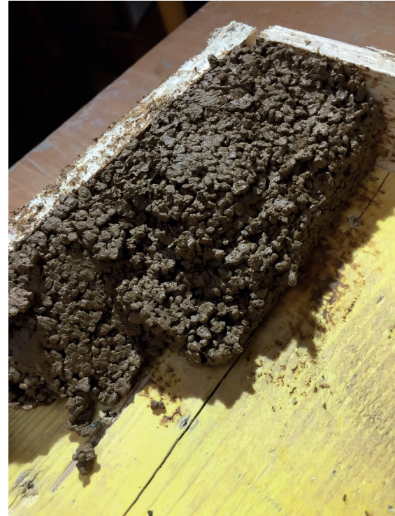
Figure 166, 167 (left) and 168 (above). Preparation and casting of sample 1. First the earth is mixed with water, then the crushed olive pits are added.
