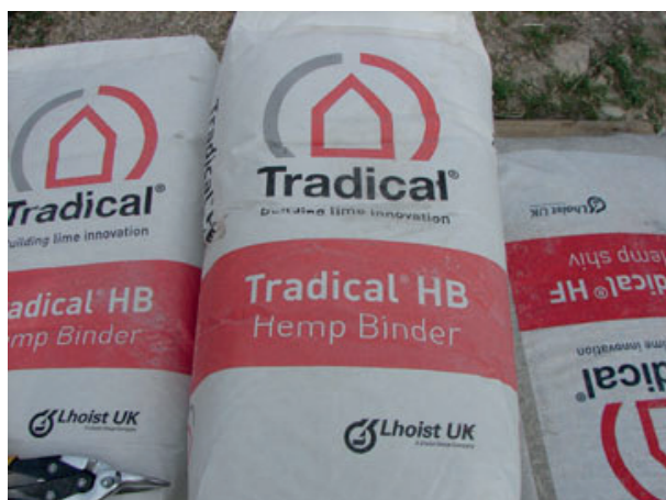
Figure 110. The Tradical specific hemp binder produced by Lhoist UK.
