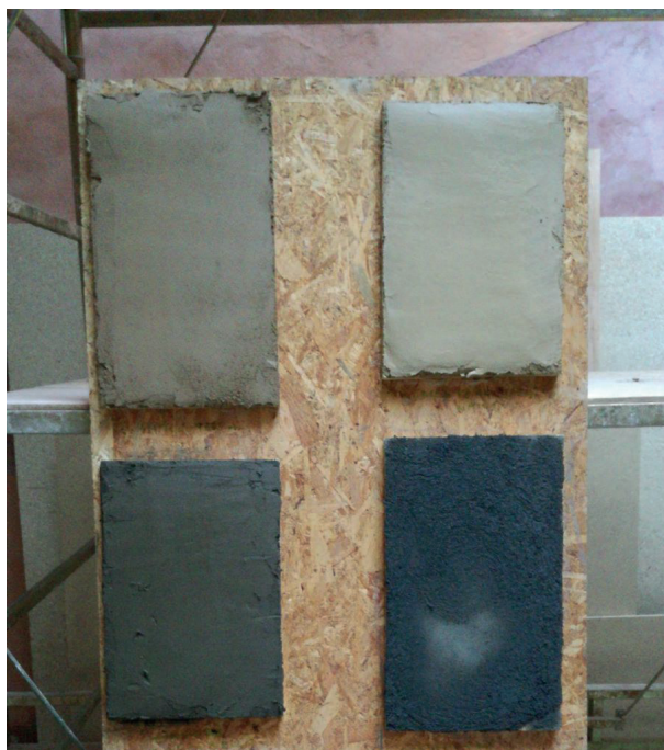
Figure 212. The charcoal plaster samples. On top on the left the plaster with 10% of char consistency. On top on the right a sample with no char addition for comparison.
