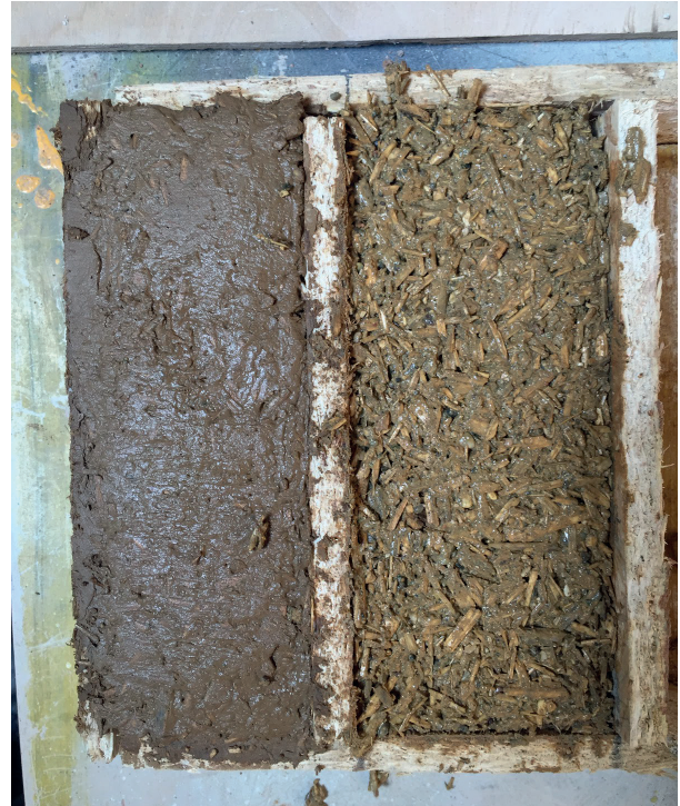
Figure 117. The two earth-hemp shiv samples, on the left earth from unfired bricks and on the right earth from subsoil
