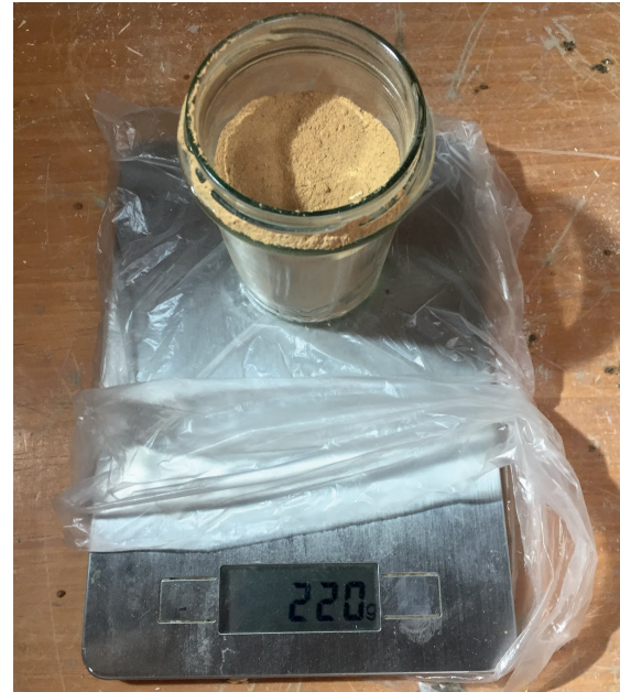
Figure 171. Earth binder from subsoil in a powdered state.
