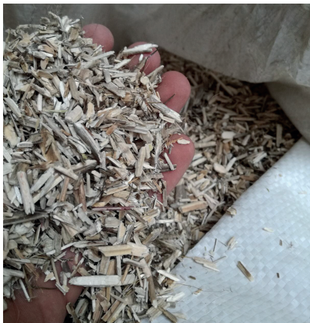
Figure 109. The hemp shiv donated from Assocanapa. The gray colour is due to the presence of dust and excessive fibers. Photo: Andi Dani
