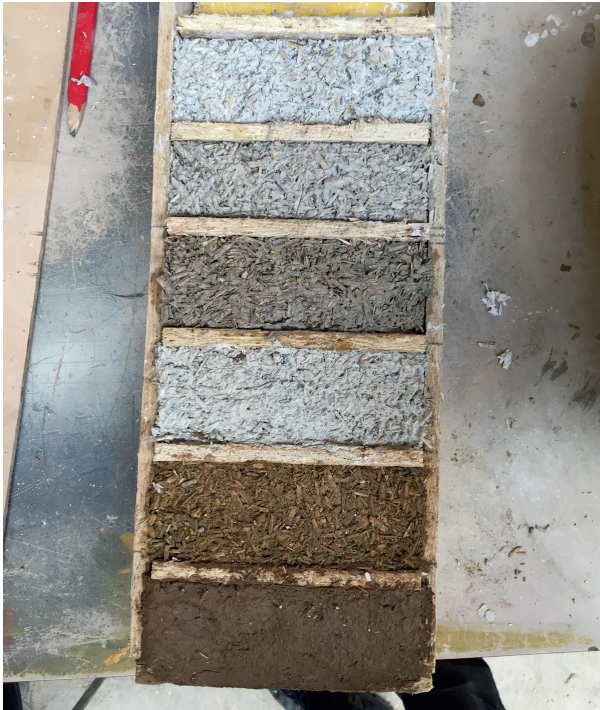
Figure 131. The created samples inside the woodform. The lime putty and milk mix on top. Photo: Andi Dani
