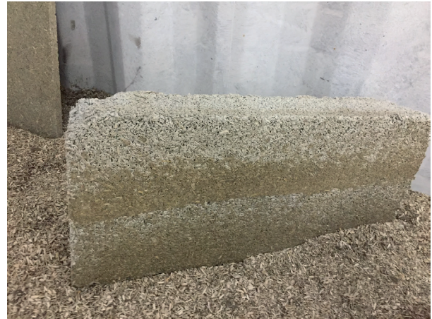
Figure 132. The sample of lime putty, milk and egg white exhibited at the Canapissima hemp fair. Photo: Andi Dani
