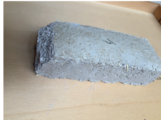
Figure 184. The dry sample 4. The brown stains on the top surface derive from the remaining oil in the olive pits. Photo: Andi Dani
