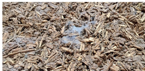
Figure 158. Mold manifestation on drying hempcrete. Photo:Andi Dani
