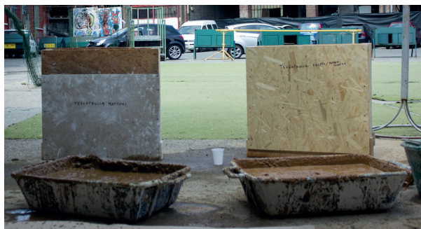
Figure 81. The two 60 \times 60 \times 10 \text{ cm} straw clay samples built for the hot plate test. On the left the sample with subsoil clay binder and on the right the one with unfired brick clay binder
