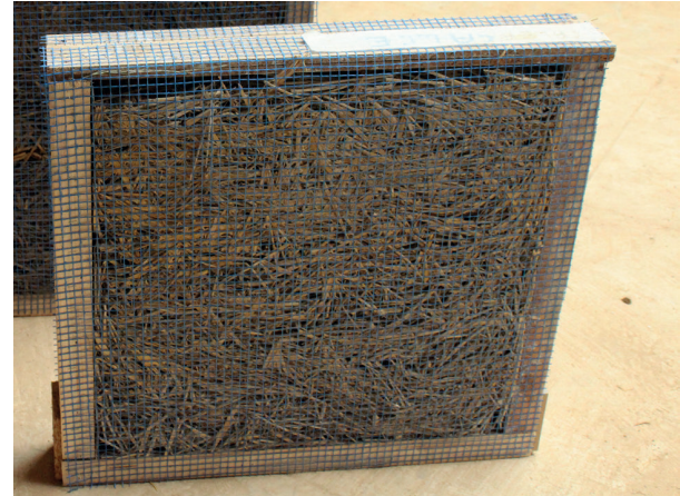
Figure 107. The 60x60x10 cm straw-lime sample, after the OSB wooden boards were taken off, in order to have a quicker and more efficient drying. A plastic grid was fixed on both sides to help preserve the shape of the sample.
