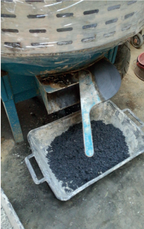
Figure 226. The mixing process was done with a rotating mill. Photo: Andi Dani
