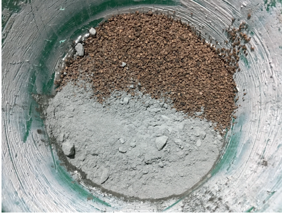
Figure 196. Preparation of sample 7. Portland cement and crushed olive pits are first mixed while dry, then water is added.
