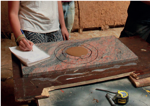
Figure 66. Testing if the clay slip is ready, pouring it into a flat smooth surface and checking if it spreads in a 15 to 20 cm radius. Photo: Margherita Pagliari
