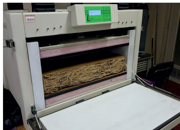
Figure 105. The straw-lime sample inside the Lasercomp FOX600 machinery before the initialization of the analysis.
