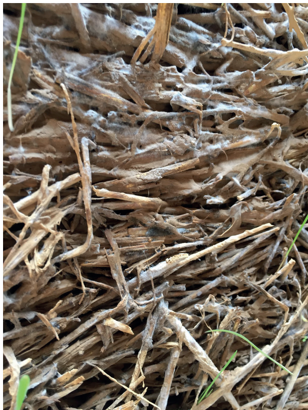
Figure 80. Mold and vegetation manifestation during the drying process of the straw and clay insulation. This phenomenon is normal. Usually the builders know they can start applying finishing layers once the vegetation is all dried up and dead.
