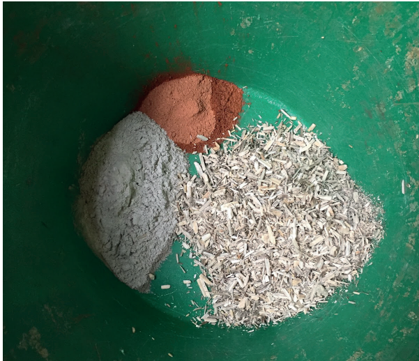
Figure 137. The dry ingredients of the cocciopesto-NHL 5-Hemp shiv sample.
