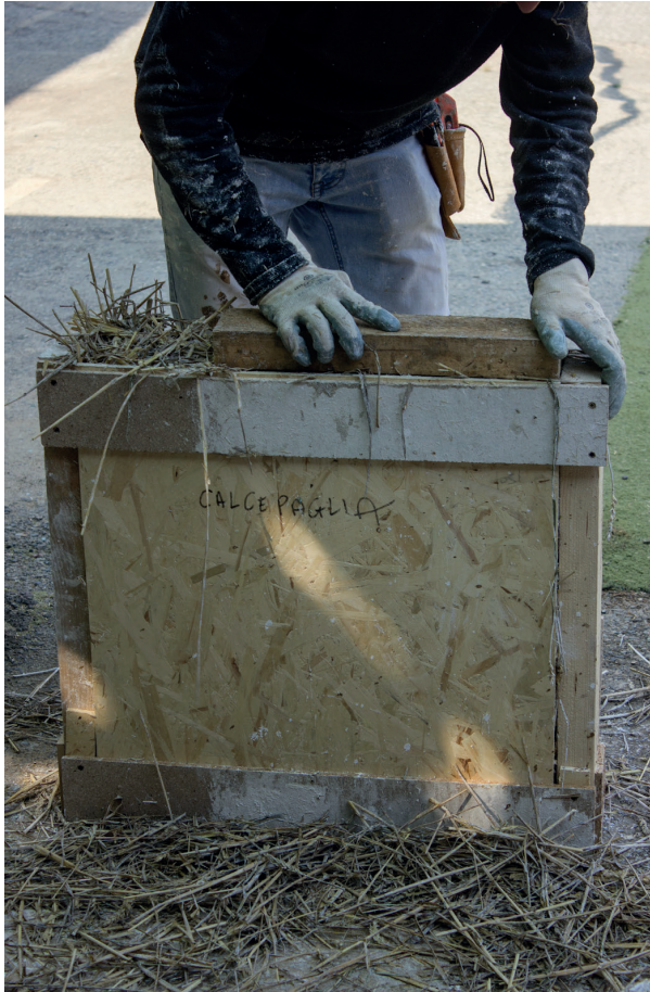
Figure 106. The preparation of the straw-lime sample which was sent in the laboratory for the Hot Guarded Plate test.
