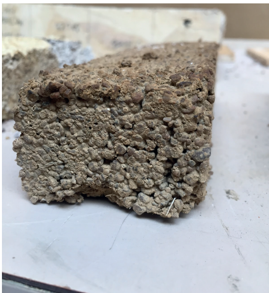
Figure 174 and 175. Dried sample 2. Very few oil stains can be seen.
