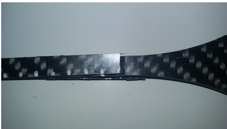
Figure A.8: Close view of fracture for specimens of groups D.
