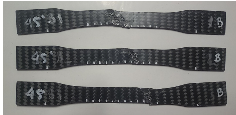
Figure A.3: Failed specimens of group B.
