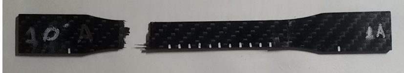
Figure 5.7: Failed specimen of group A.
