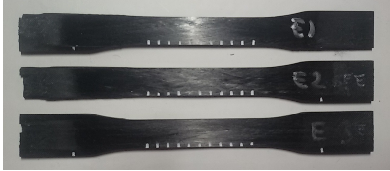
Figure A.9: Specimens of group E after testing. None of the specimens has failed in the gage section.
