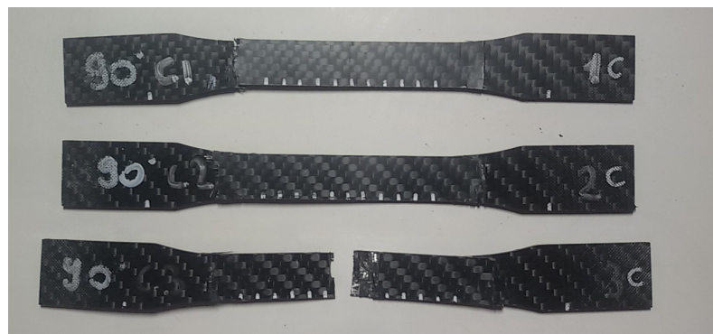
Figure A.5: Failed specimens of group C.
