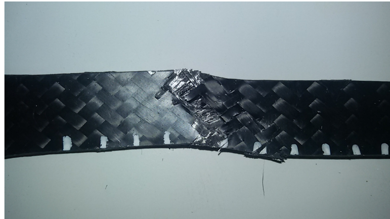
Figure A.4: Close view of fracture for specimens of groups B.
