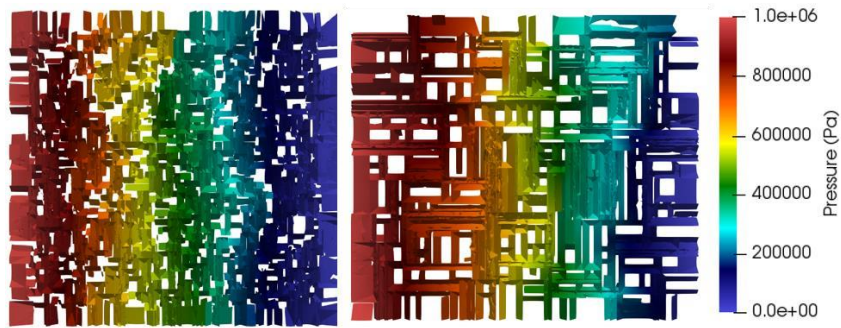
Figure 2: Pressure propagation for 2 sets of fractures with same density and 2 different c values
