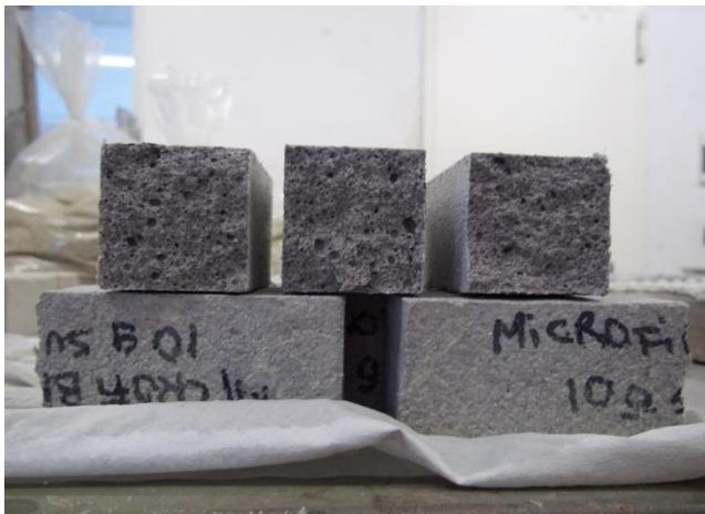
Figura 106 Provini BETON P16 + microfibre L/C
