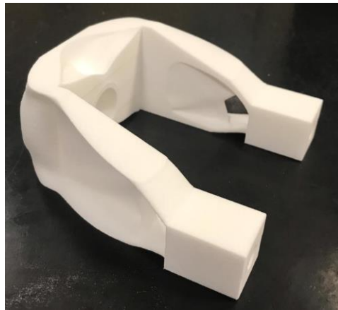
Figure 13: 3D Printed part modeled by SolidThinking Inspire
