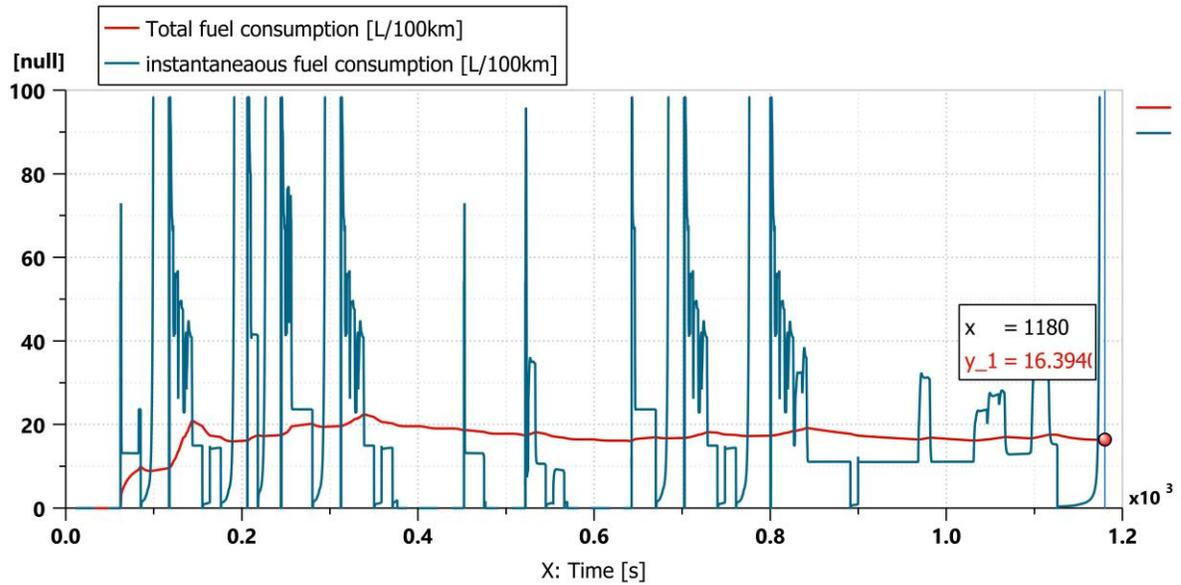
Figure 6.3: total and instantaneous fuel consumption for P2 configuration
