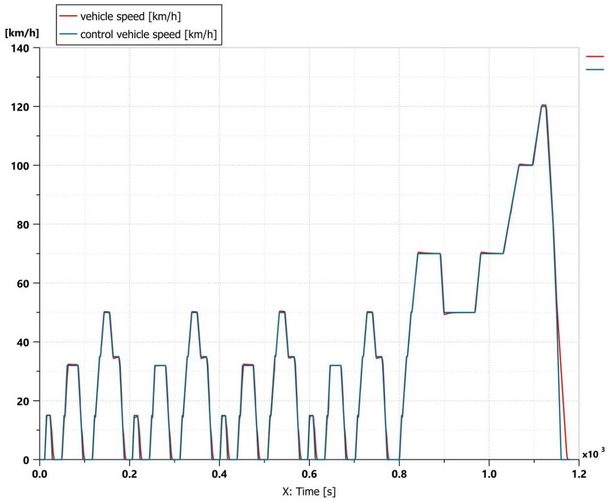
Figure 6.1: vehicle speed and control speed for P2 configuration.
