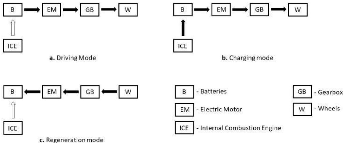
Figure 2.2: Architecture and Power-flow in a series hybrid vehicle
