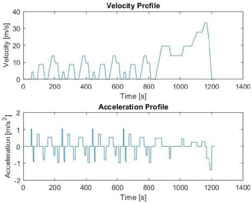
Figure 4.6: velocity and acceleration profiles in NEDC
