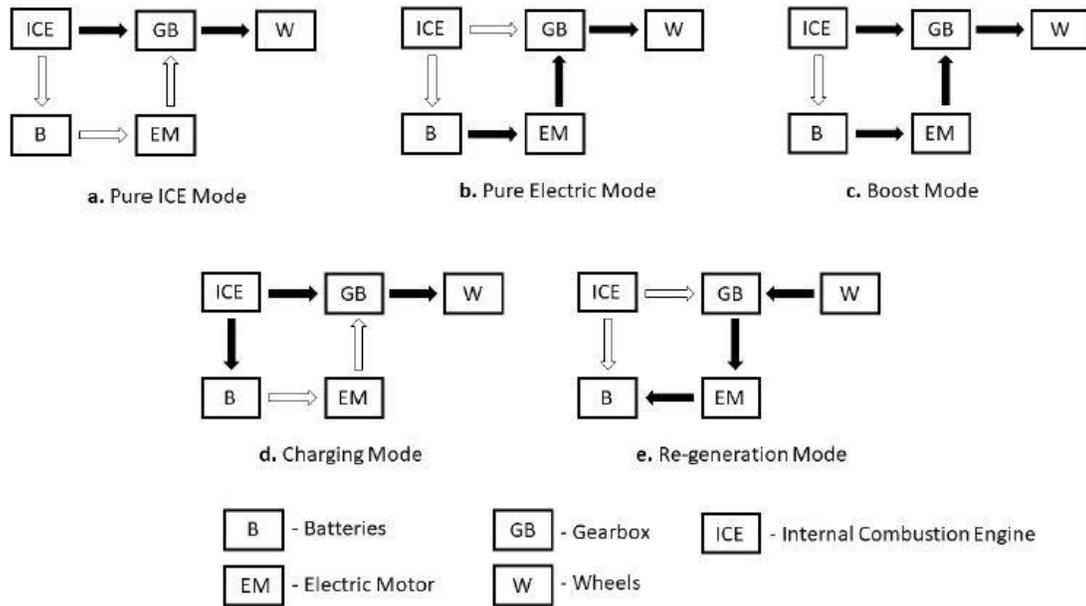
Figure 2.3: Power-Flow in a parallel hybrid vehicle
