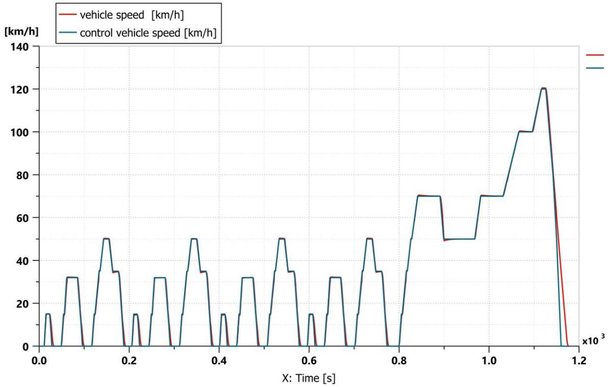
Figure 6.4: vehicle speed and control speed for P3 configuration.
