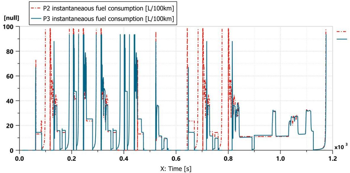
Figure 6.9: instantaneous fuel consumption for both configurations
