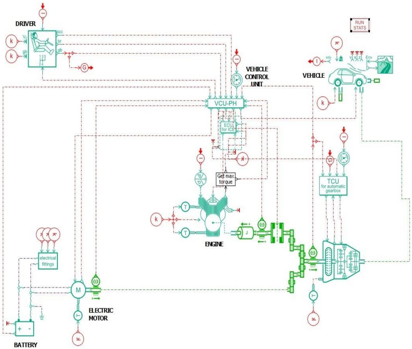
Figure 5.1: P2 hybrid configuration
