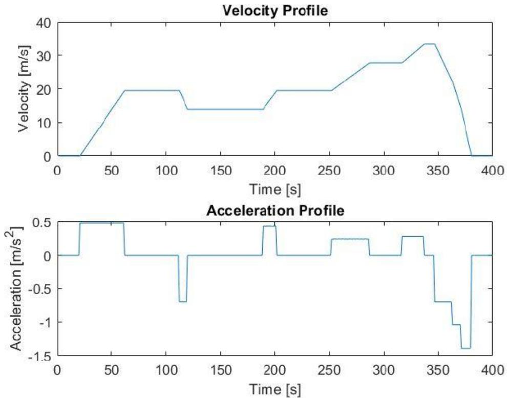
Figure 4.5: velocity and acceleration profiles in EUDC
