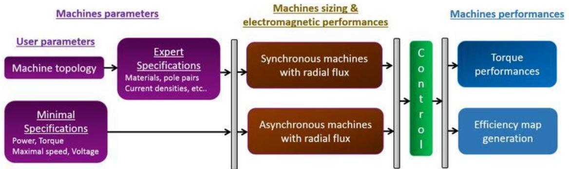
Figure 4.10: electric machine performances diagram
