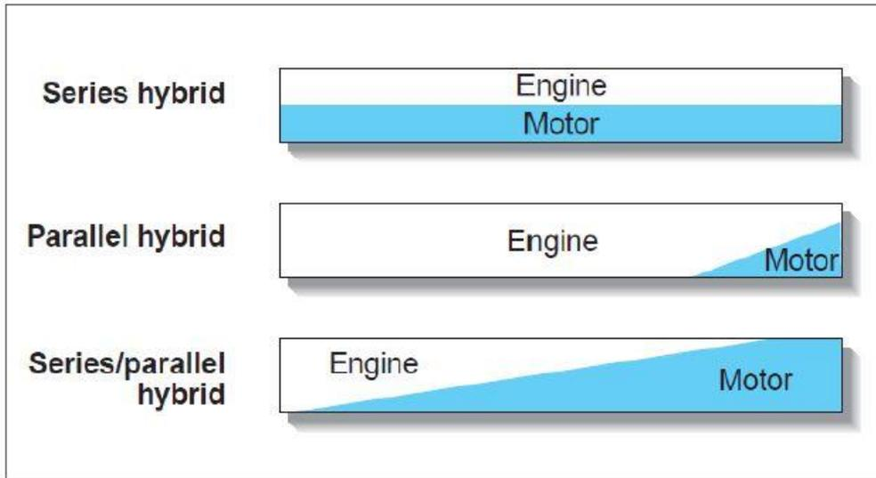
Figure 2.6: ratio of engine and motor operation in hybrid systems
