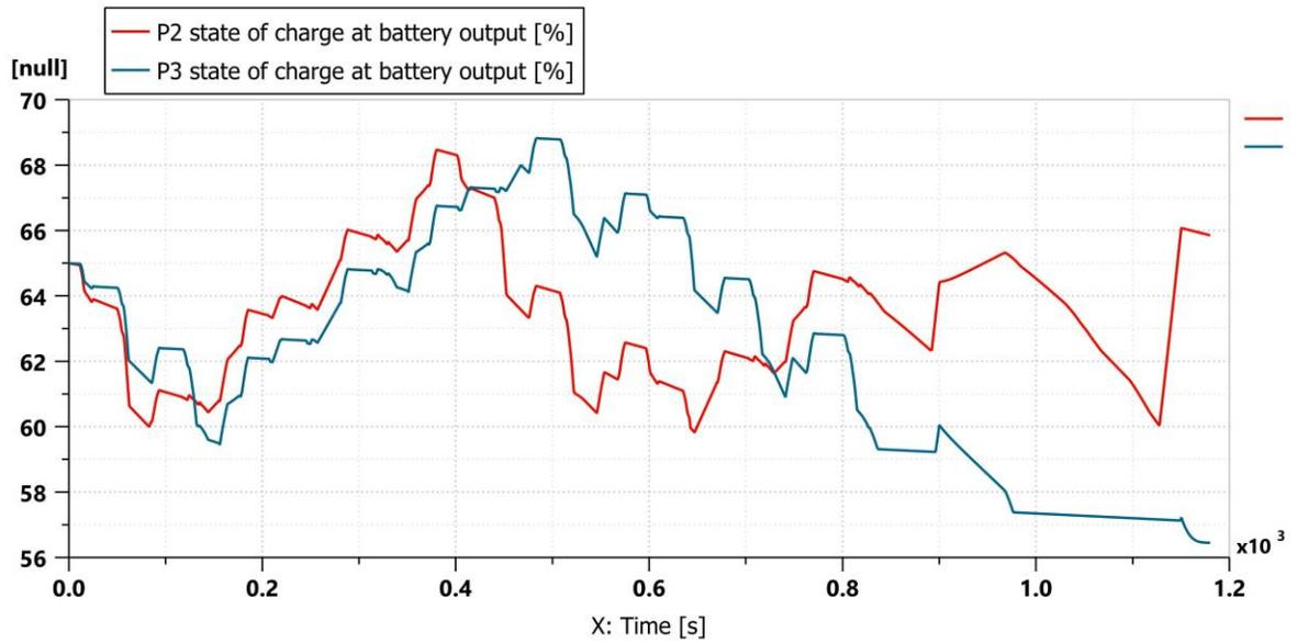
Figure 6.10: state of charge at battery output for both configuration
