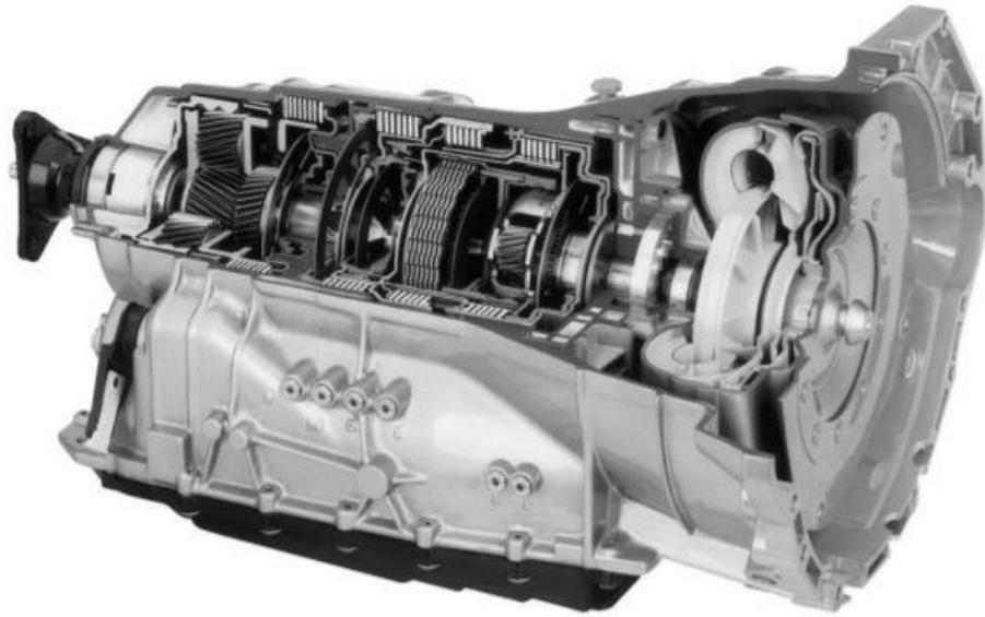
Figure 4.2: 6HP28 Automatic Transmission [7]
