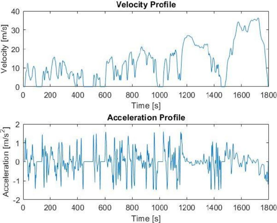
Figure 4.4: velocity and acceleration profiles in WLTP: Class 3
