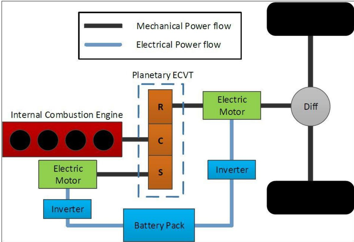
Figure 2.4: Power-Split Hybrid Powertrain Architecture
