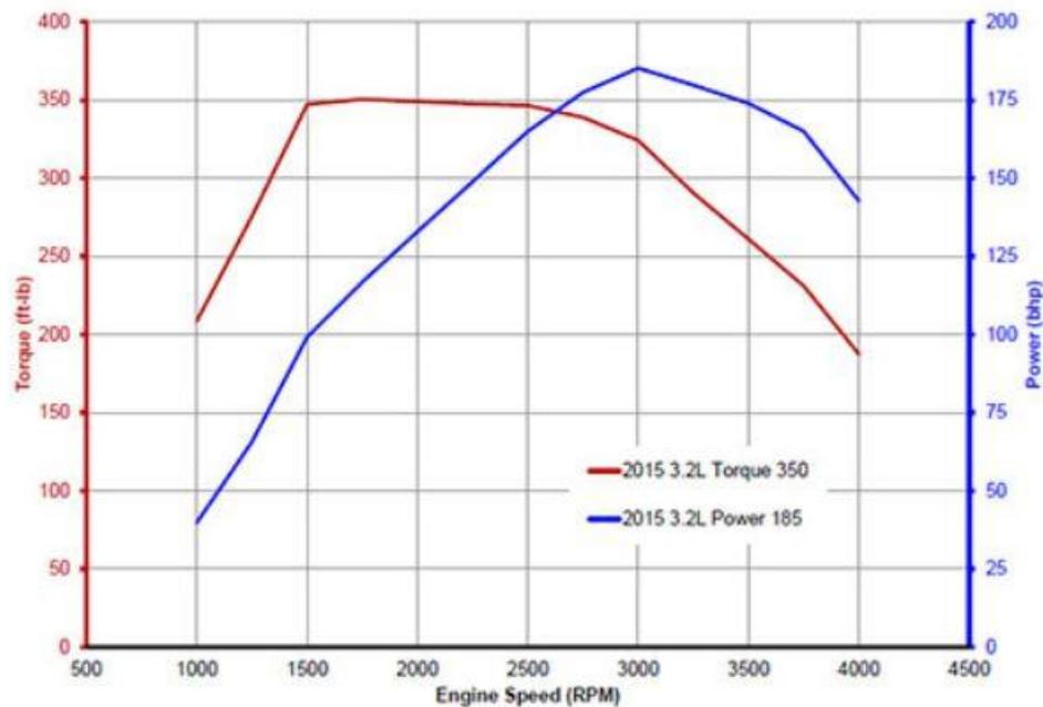
Figure 4.1: 3.2L POWER STROKE HORSEPOWER/TORQUE CURVES [6]
