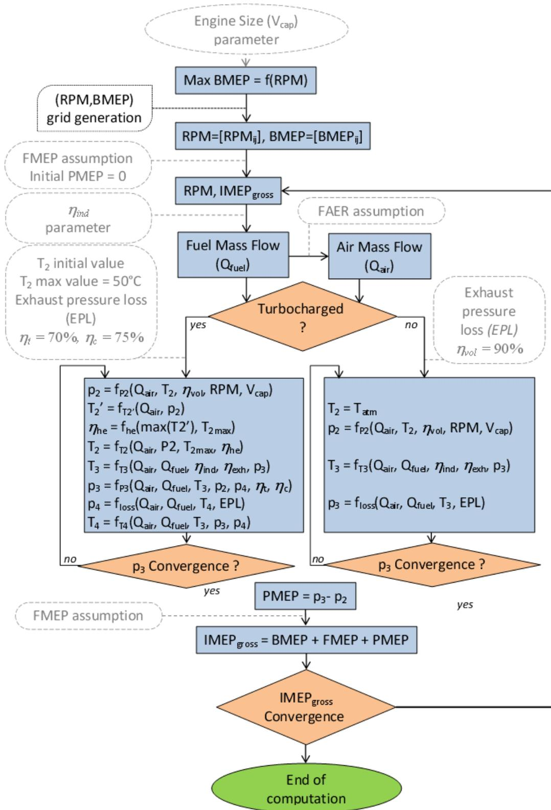
Figure 4.8: computation diagram for creating ICE data [9]
