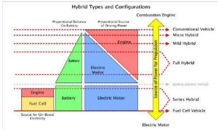
Figure 1.1: HEV classification based on level of hybridization [3]
