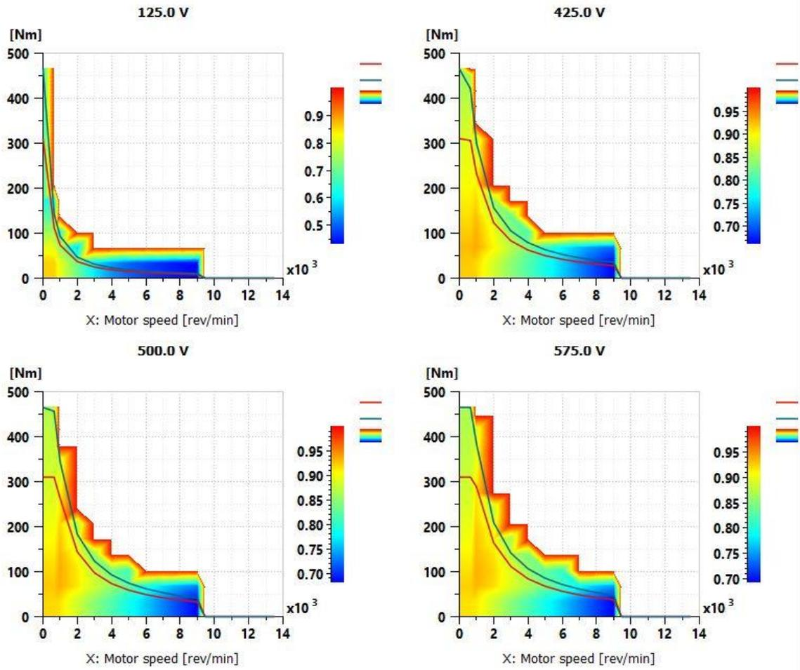
Figure 4.12: Efficiency for considered electric motor
