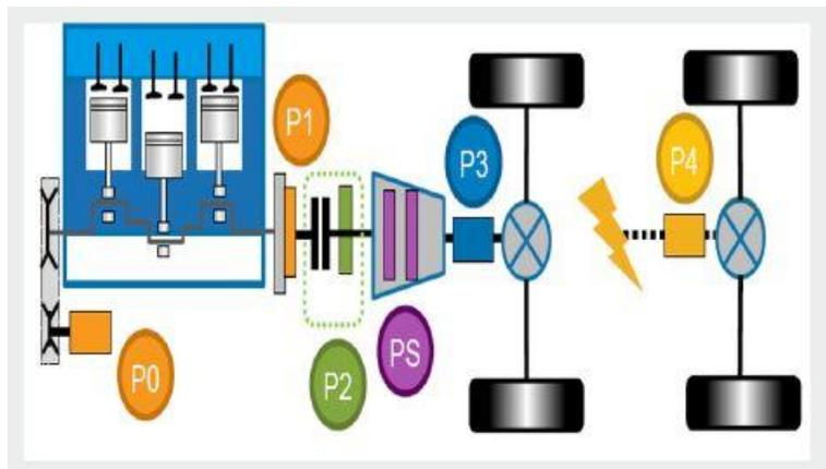
Figure 2.5: hybridization architecture based on electric motor position
