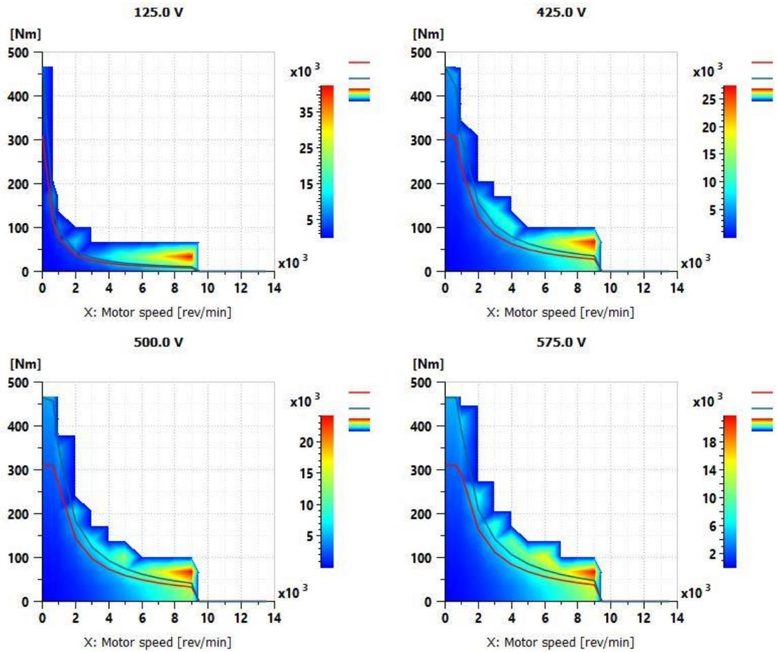
Figure 4.11: losses for considered electric motor
