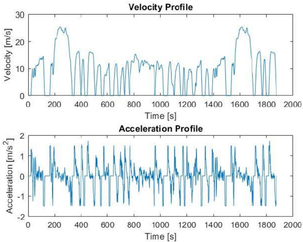
Figure 4.7: velocity and acceleration profiles in FTP-75
