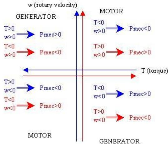
Figure 4.9: different operating modes of the electric motor/generator
