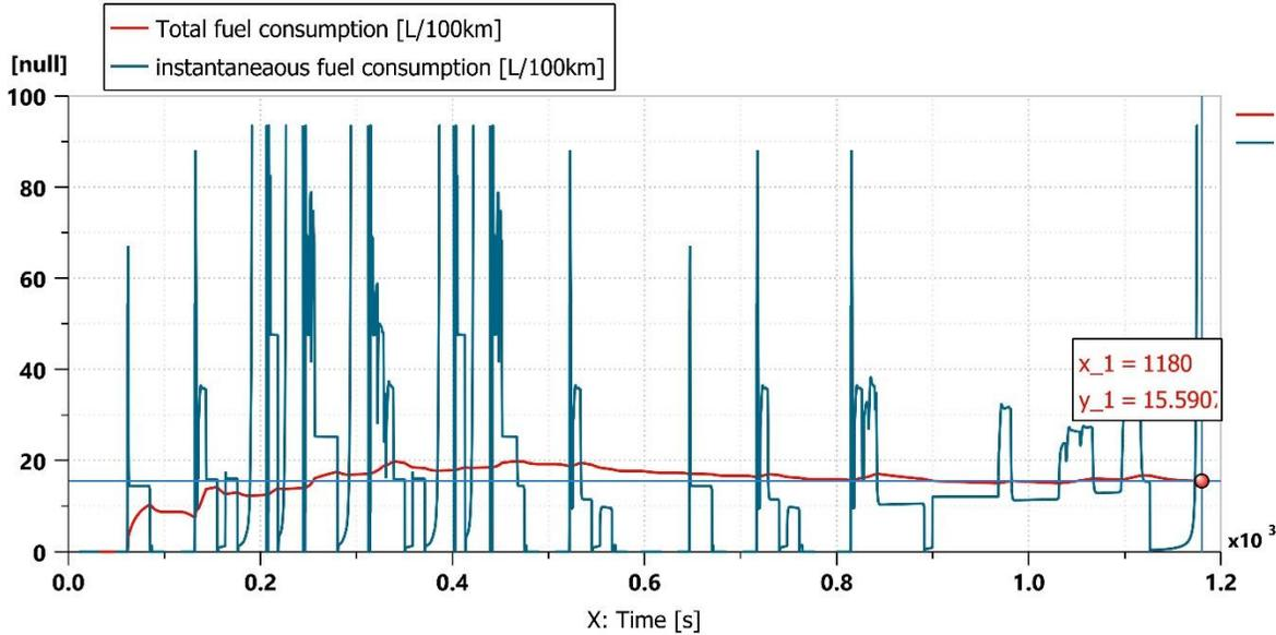
Figure 6.6: total and instantaneous fuel consumption for P3 configuration
