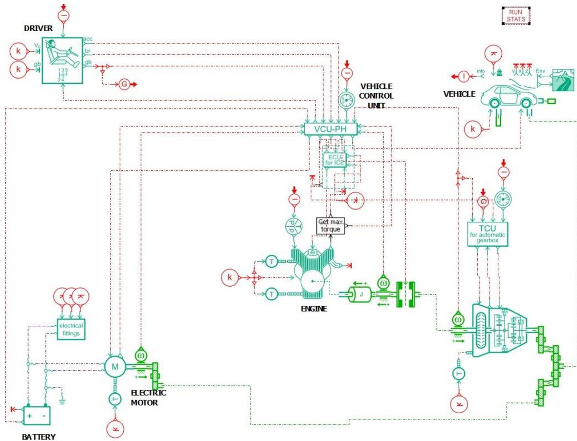
Figure 5.2: P3 hybrid configuration
