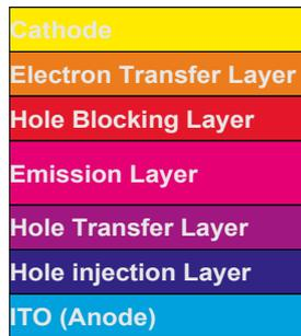
Figure 1.12: An example of multi-layered OLED structure.
