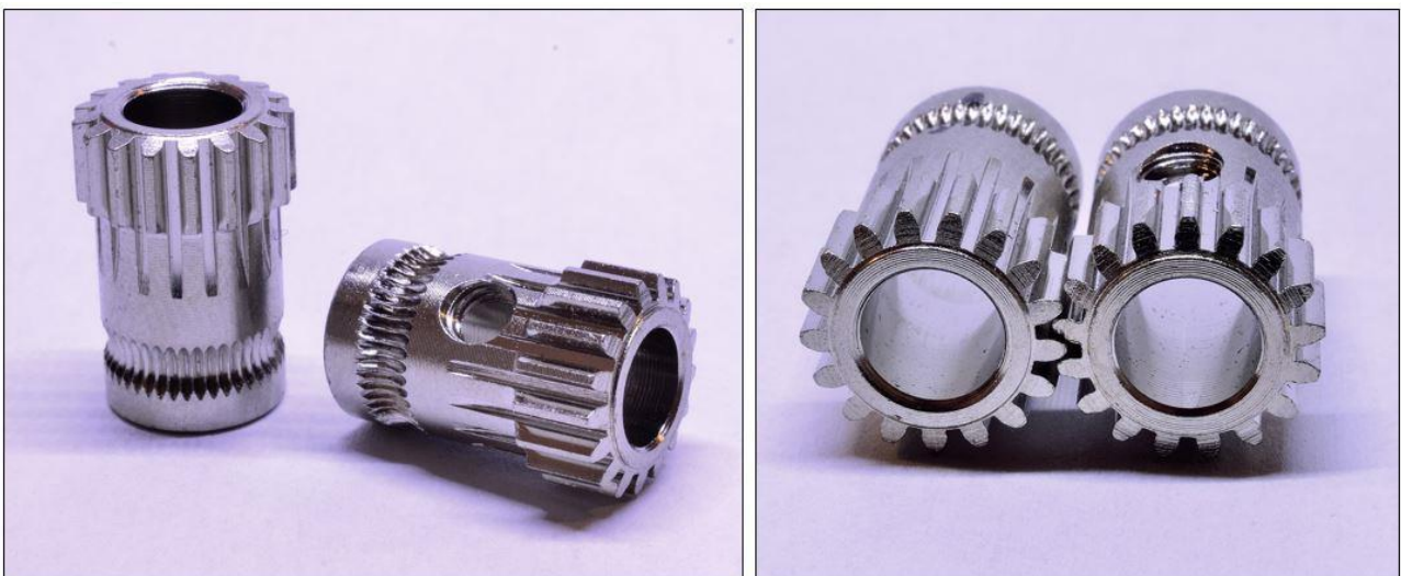
Figure 24: Extruder's Gears: the gear on the right can be screwed on the motor shaft and transmits motion with the spur gear teeth at its end to the gear on the left, the driven gear. Filament is gripped thanks to the rounded grooves on both gears
