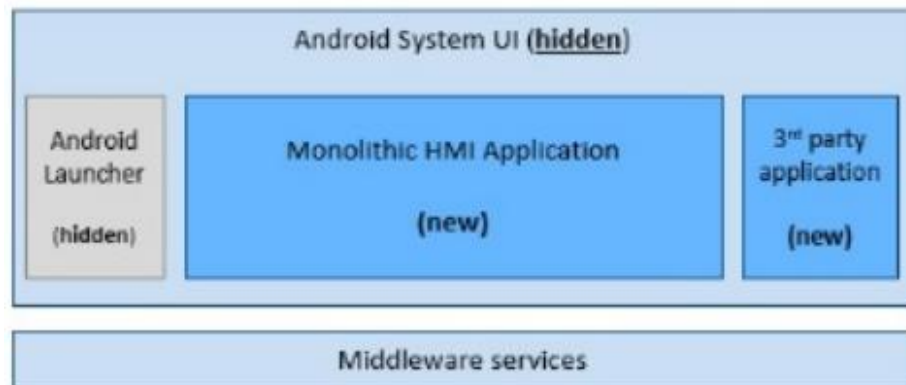
Figure 11. Android HMI Monolithic architecture
