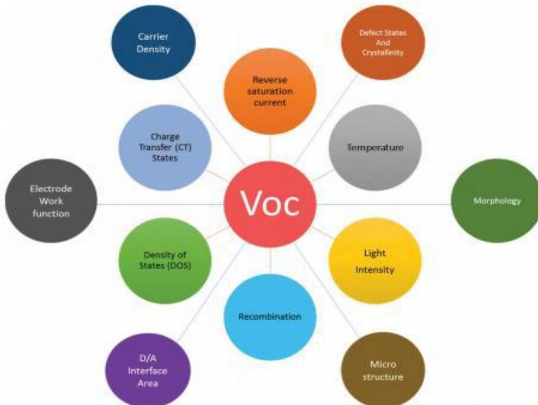
Fig. 47 Factors influencing the open circuit voltage ( $V_{OC}$ ) in organic solar cells. Each parameter influences the  $V_{OC}$  either directly or indirectly via interrelated dependencies among them. Inner circles presents direct or most influencing factors while the outer ones manifest indirect and less significant factors dependent  $V_{oc}$  [38].
