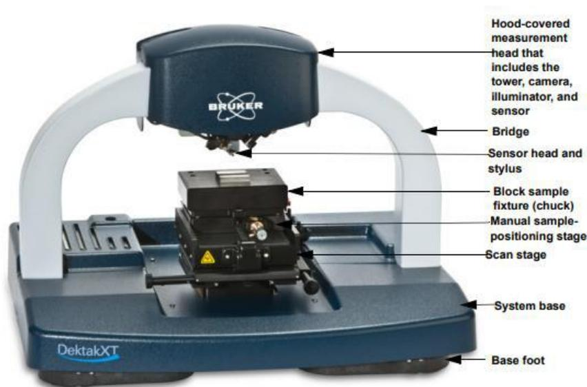
Fig. 20 DektakXT® stylus profiler tool where main parts are clearly indicated with arrows [22]
