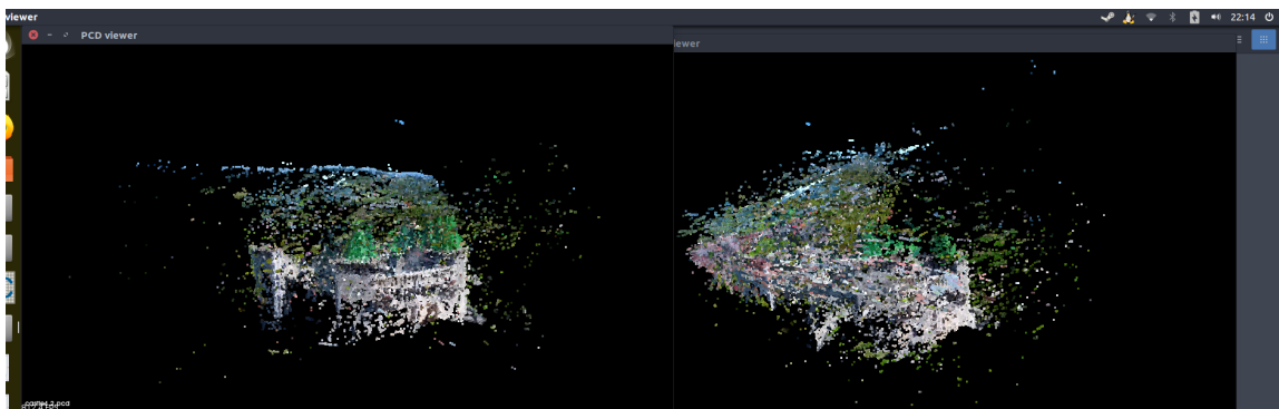
Figure 5.13: castle case:compare between original SLAM(right) and CNN depth estimation SLAM(left) 2
