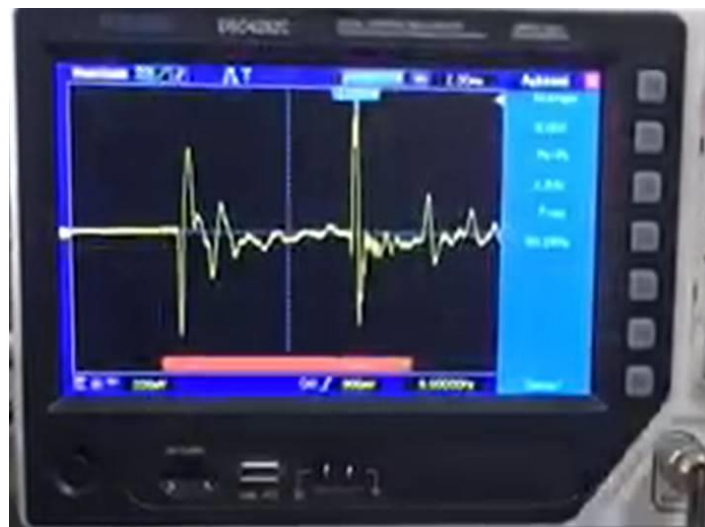
Figure 4-11 Real waveform of the knock sensor
