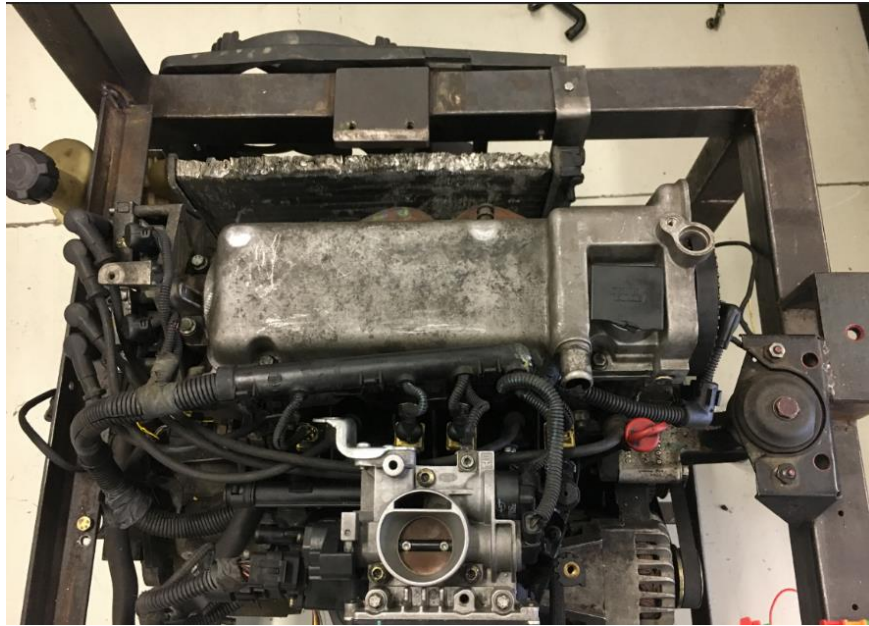
Figure 4-46 Engine body fixes on the test bench
