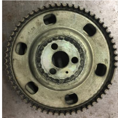
Figure 4-25 Crankshaft reluctor wheel with 2 missing teeth
