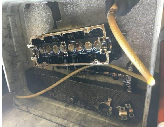
Figure 4-2 Clean the stubborn oil pollution with air pressure and gasoline
