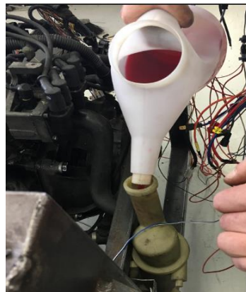
Figure 6-4 Inject the coolant oil in the engine
