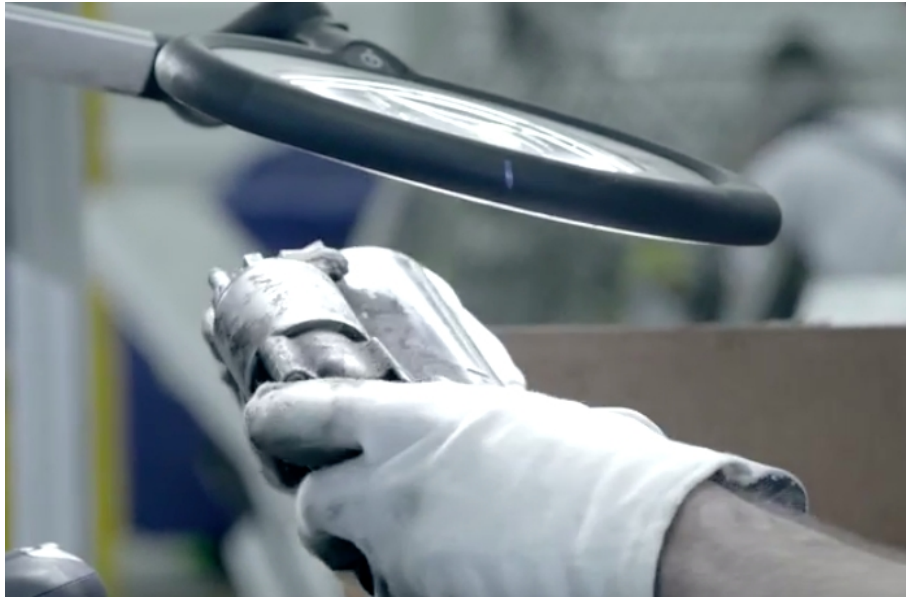
Figure 19: A recovered core is subjected to a detailed inspection from a Bosch operator.
