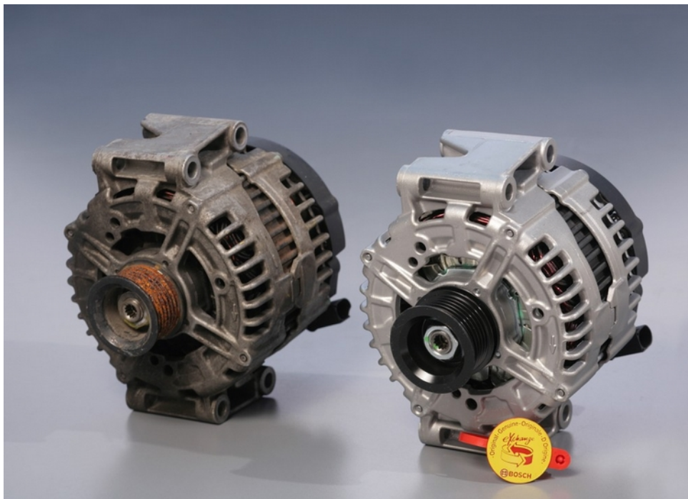
Figure 11: Bosch eXchange product. Old and remanufactured Bosch Rotating Machine.
