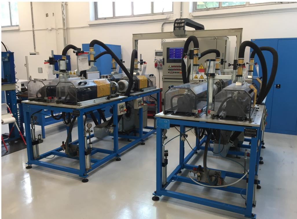
Figure 4.4: Test rigs for balls bearing tests
