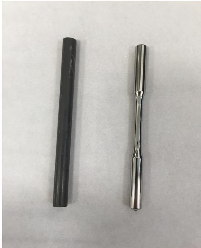
Figure 4.1: Raw steel coil cut and final specimen
