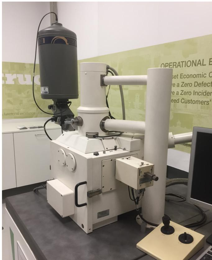
Figure 4.6: Scanning Electron Microscope
