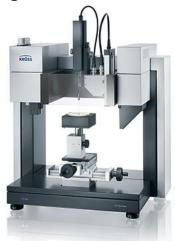
Figura 4.6: Drop Shape Analyzer 100 [8]
