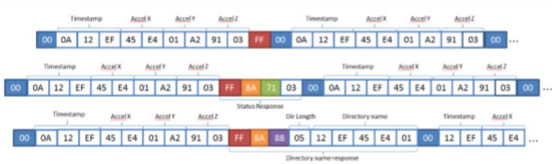
Figure 4.6: How the data are stored inside the Shimmer2R [67]
