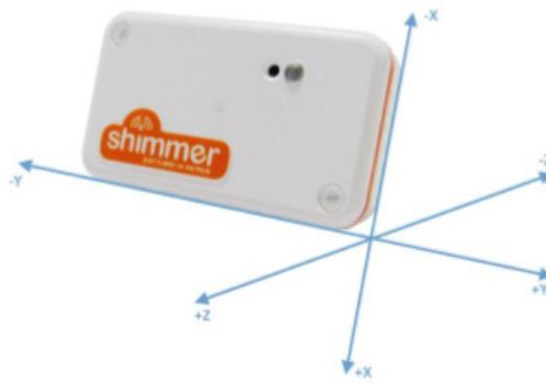
Figure 4.4: The system of acceleration of the Shimmer [66]
