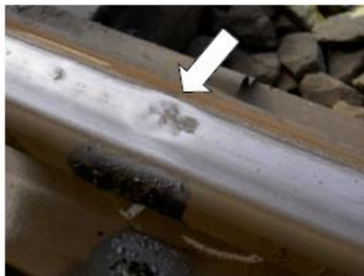
Figure 11: Damage due to pressure after a long time in the track.
