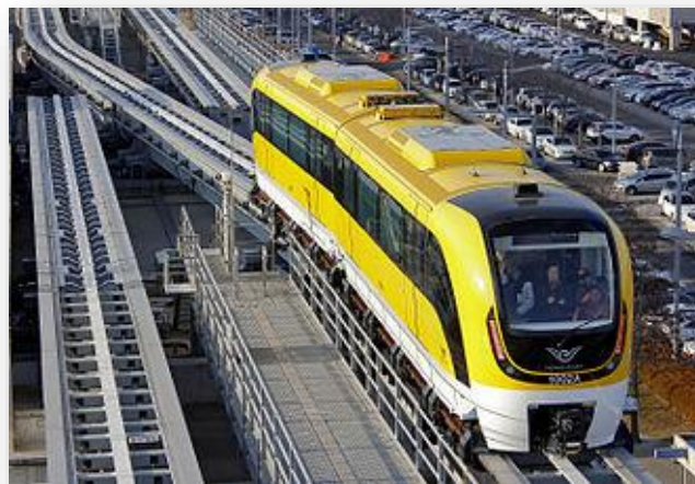
Figure 21 ECOBEE, it adopts EMS system with Iron-cored long stator LSM [31]
