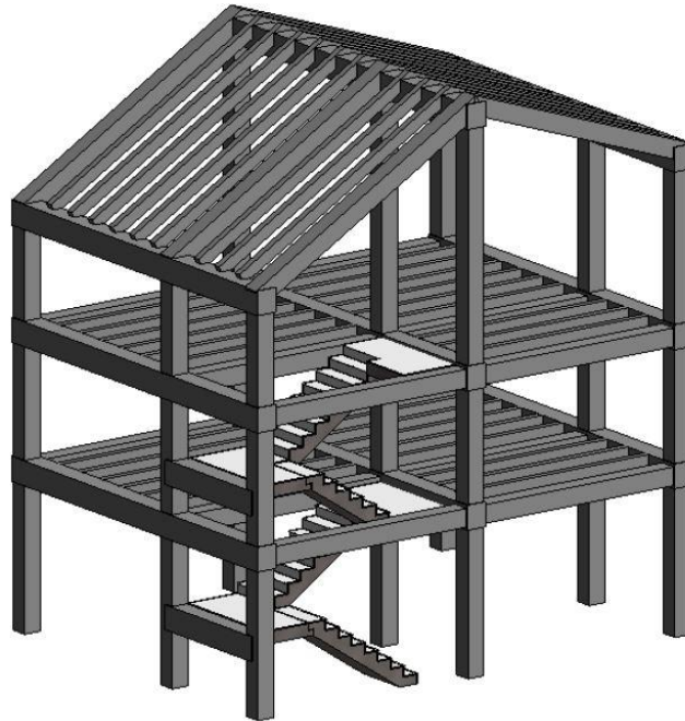
Figure 5.5 - Structural skeleton of the building (Revit 2018)
