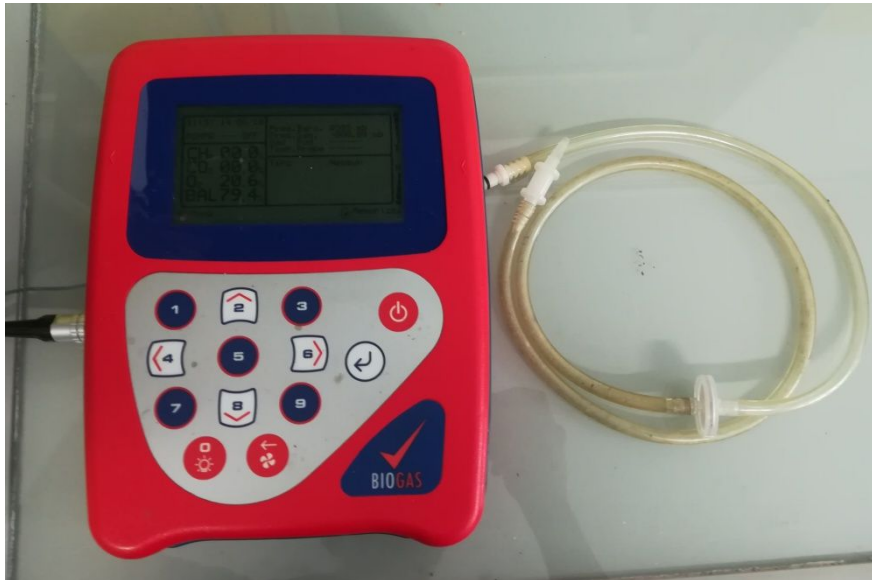
Figura 3: Geotech Biogas 5000 Portable Biogas Analyser.
