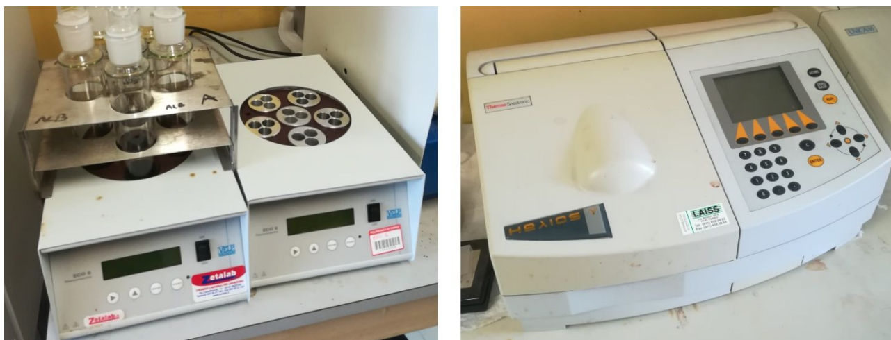
Figura 5: VELP ECO 6 Thermoreactor (a sinistra) e Spectronis Helios Gamma (a destra).
