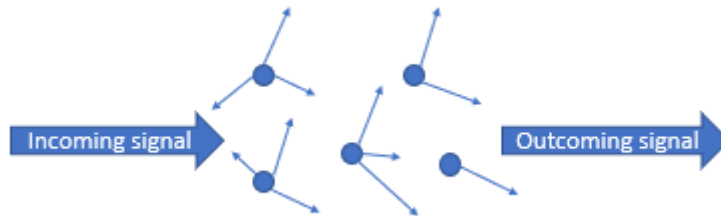
Figure 3.3. Dispersive attenuation (for scattering) [11]
