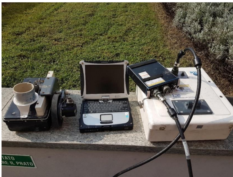
Figure 4.1. Equipment: at the left, the 900MHz antenna with the wheel odometer, in the center the computer, in the right the GPR Unit and the 200MHz antenna
