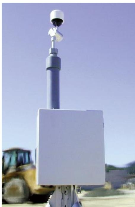
Figura 5.5-8 E-Sampler (Met One).
