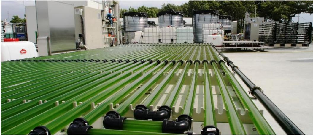
Figure 10: Horizontal tubular PBR (Picture source: [algarefinery.com](http://algarefinery.com))
