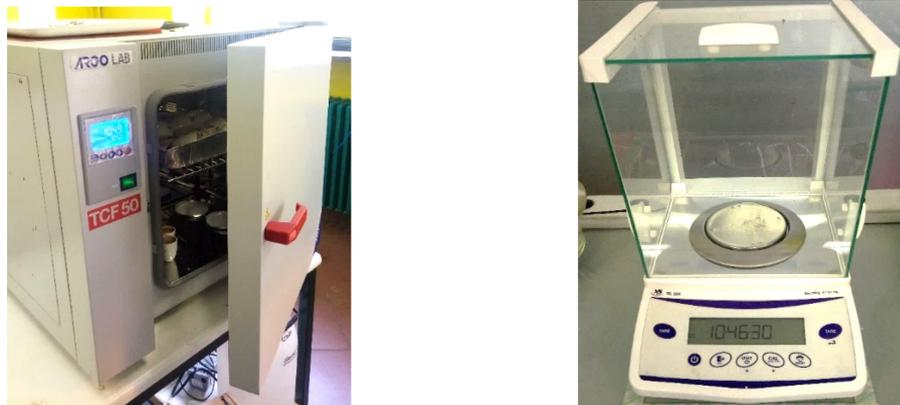
Figure 23: a) On the left, fan-assisted oven, b) On the right, analytical balance
