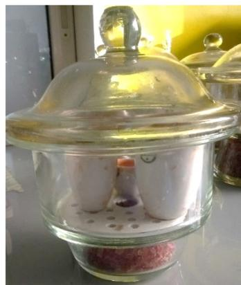
Figure 24: Desiccator with crucibles
