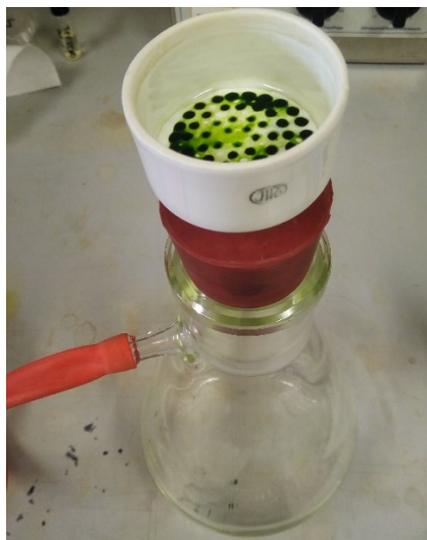
*Figure 25: Paper filter and Buchner funnel*
