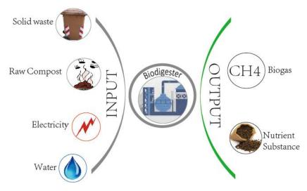
Map 56: Input - Output of Biodigester
