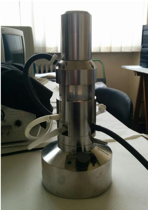
**Figure 3.** Granulometric analysis, sample container.
