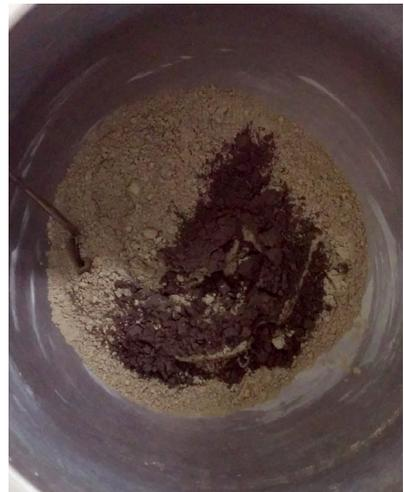
**Figure 8.** Water-superplasticizer-Biochar solution. (Left)
