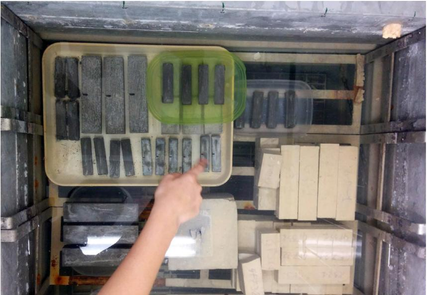
**Figure 14.** Cement pastes in curing tank.
