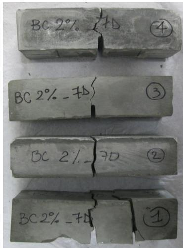
**Figure 24.** Portions of broken prisms after TPB test
