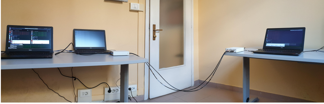
Figure 4.1: OAI testbed at Politecnico di Torino. From the left: EPC+MEC PC, eNB PC, UE PC
