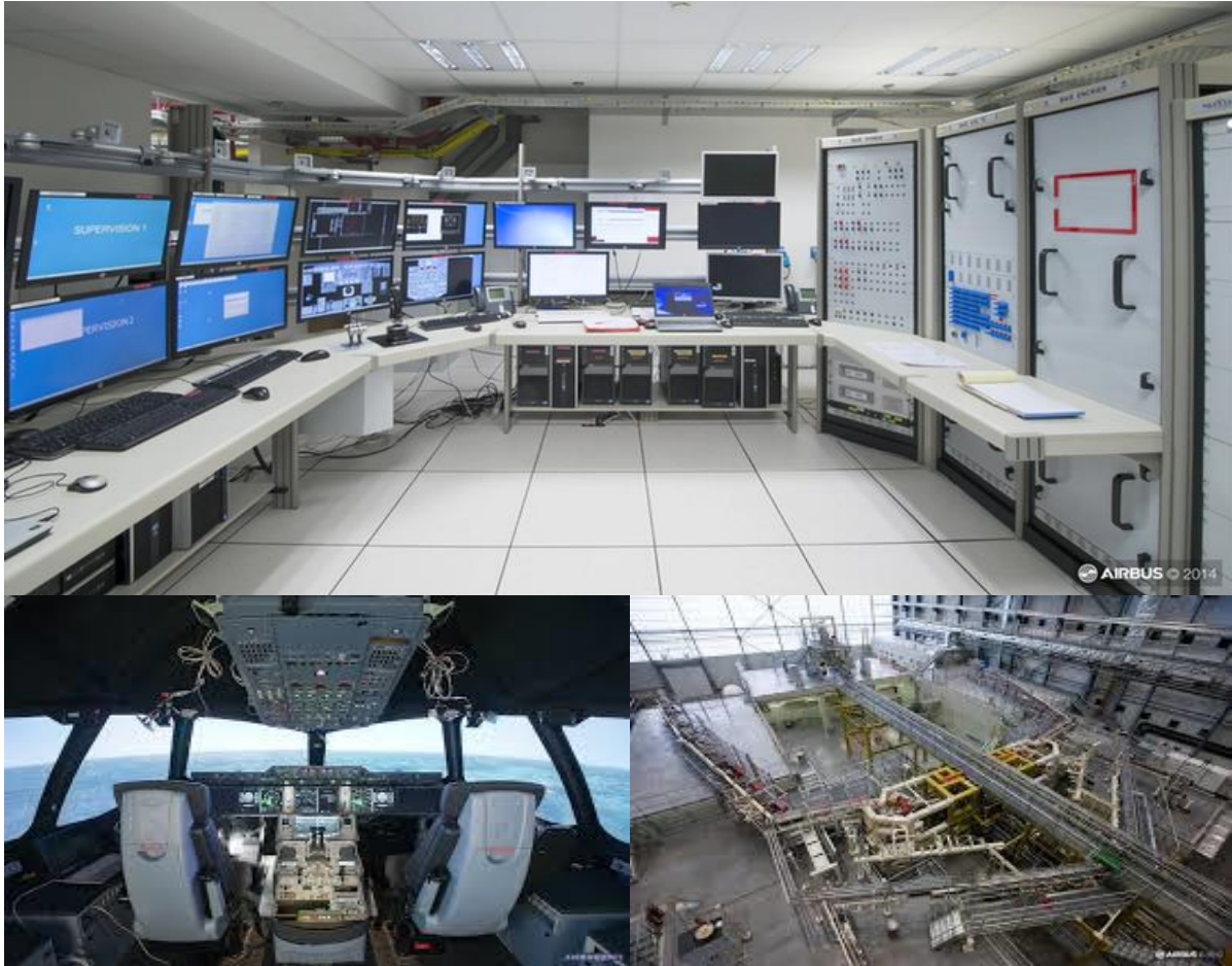
Figure 4 : testing facilities (top FIB2 NEO test bench, lower left A350 simulator and right A350 iron bird)
