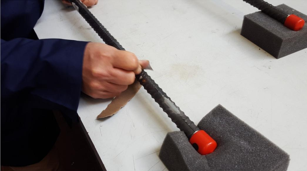
Fig. 81: Sanding off bar's surface
