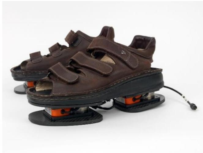
**Fig. 1.11** Xsens Forceshoes are very accurate, on the other hand they are bulky and expensive
