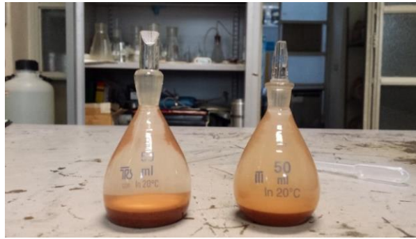
Figure 16: pycnometers filled with the grain material and distilled water
