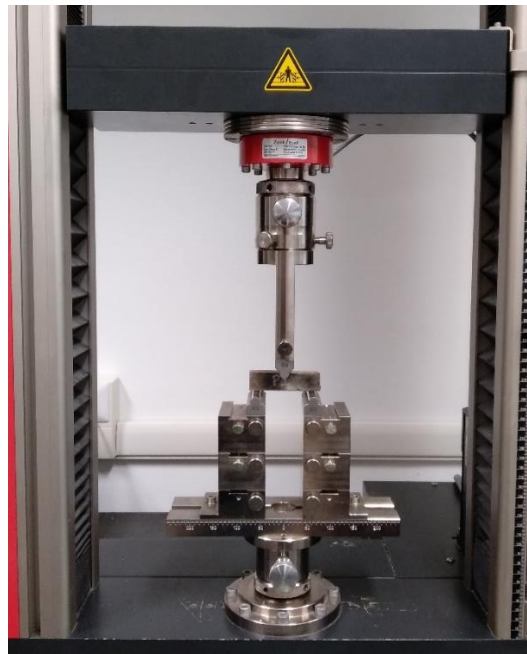
Figure 24: three-point flexural test example.
