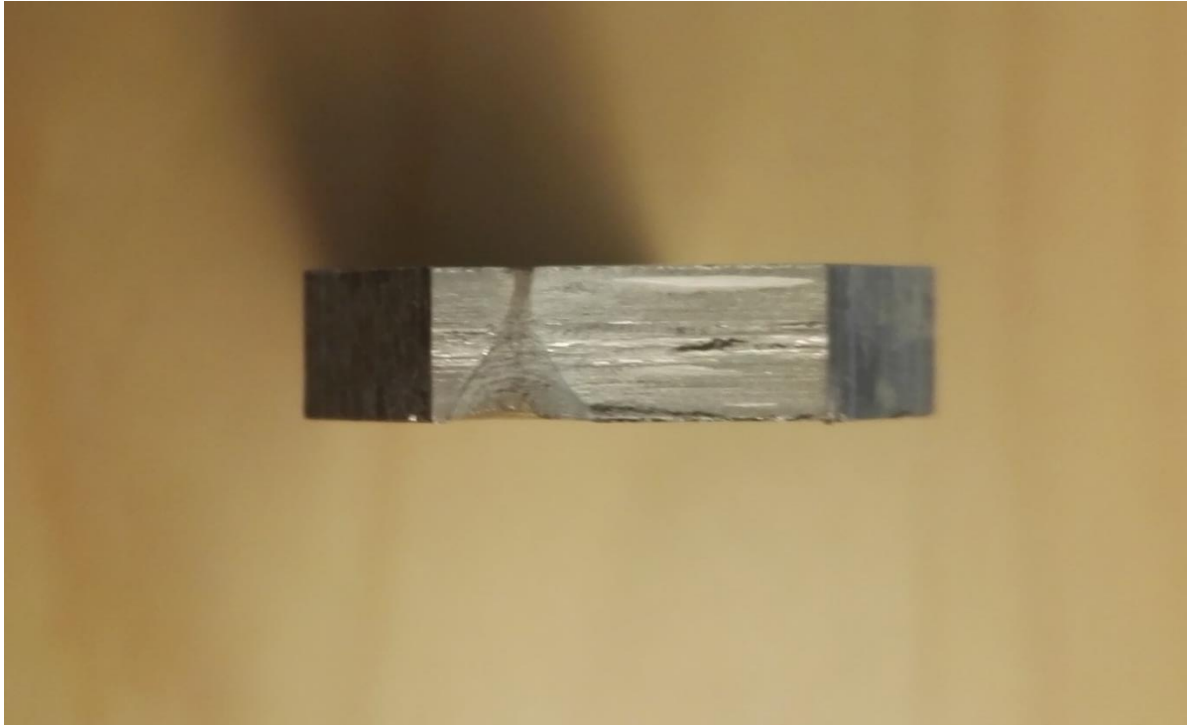
FIGURE 16 SPECIMEN 12, MAX LOAD 50 MPA, FATIGUE LIFE 511426 CYCLES, R=0
