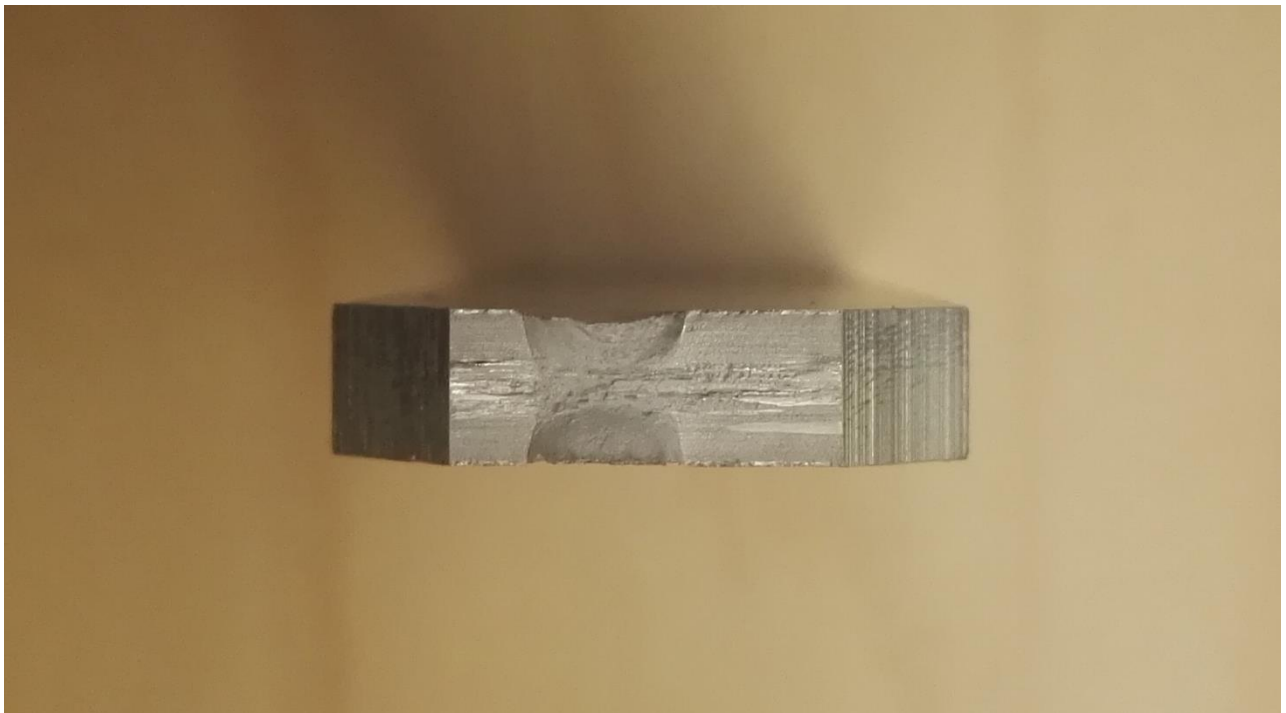
FIGURE 21 SPECIMEN 13, MAX LOAD 120 MPA, FATIGUE LIFE 116732 CYCLES, R=0.5
