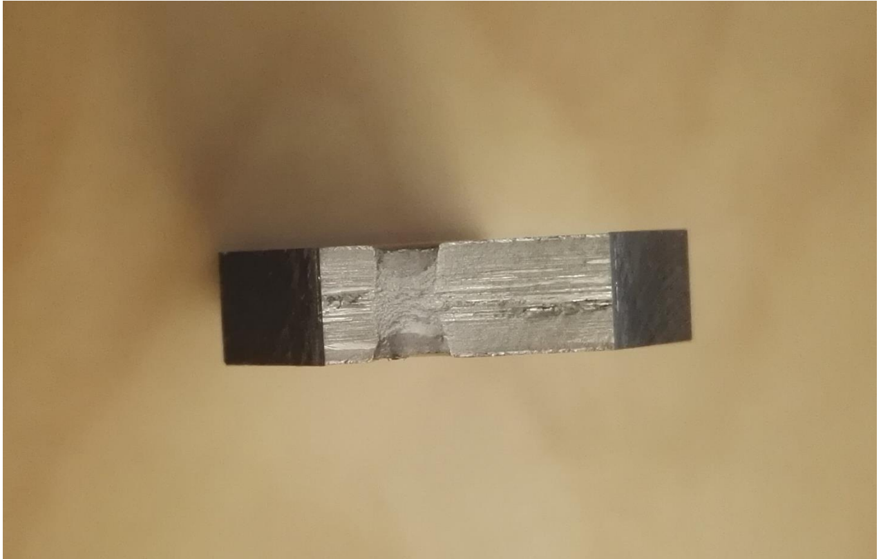
FIGURE 20 SPECIMEN 14, MAX LOAD 80 MPA, FATIGUE LIFE 653514 CYCLES, R=0.5
