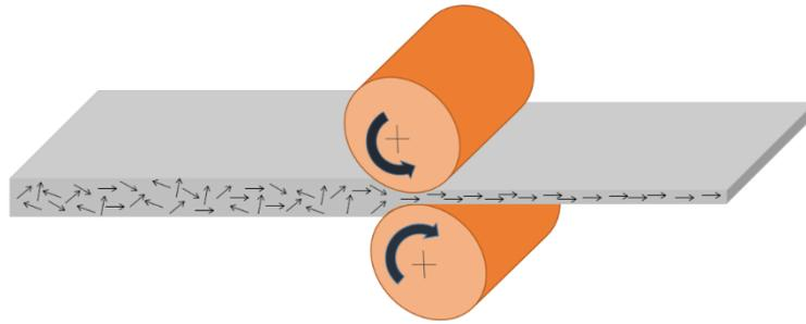
Figure 6 - Isotropy and thickness reduction in the Rolling process
