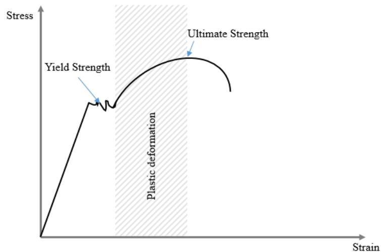
Figure 7 - Area of the materials plastic deformation
