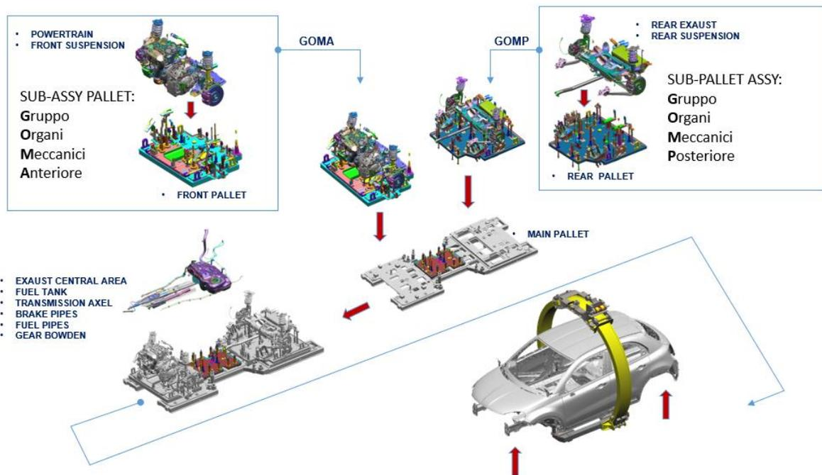
Figure 15 - Operations sequence of a Marriage process
