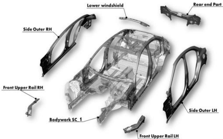
Figure 11 - Standard components of a typical BiW
