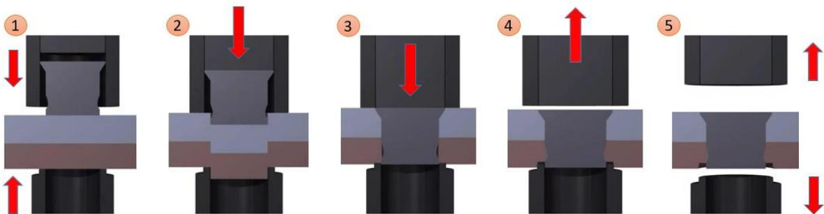
Figure 23 – Solid Punch Riveting process steps
