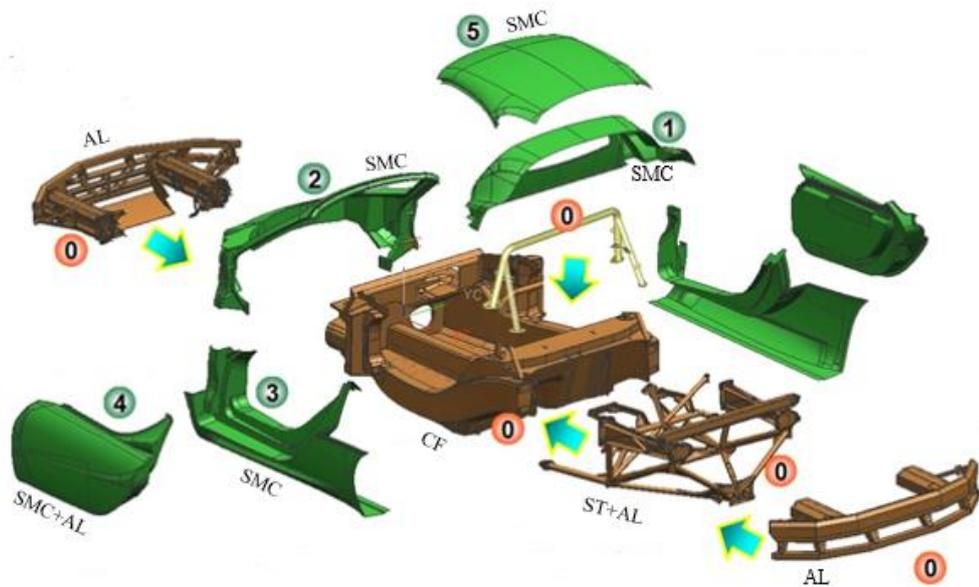
Figure 21 – Assembly sequence and different materials of the Alfa Romeo 4C chassis
