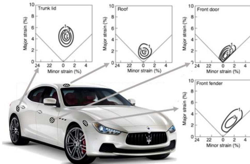
Figure 9 - Example of the formability test in automotive
