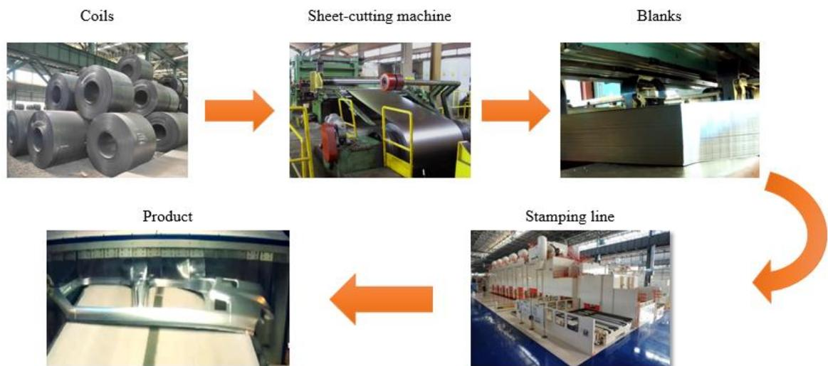
Figure 5 - Summarized scheme of the stamping process
