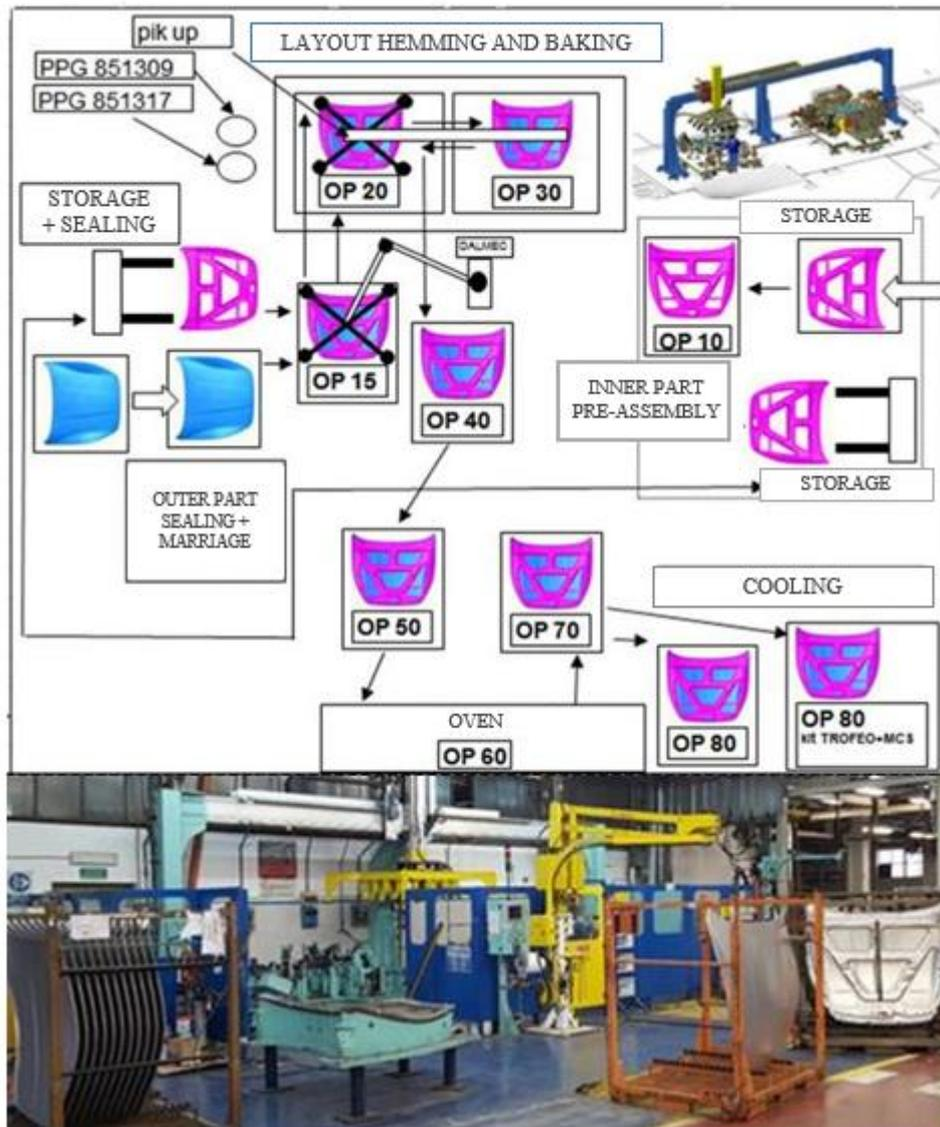
Figure 26 - Hood pre-assembly cells layout, Ex ITCA Plant
