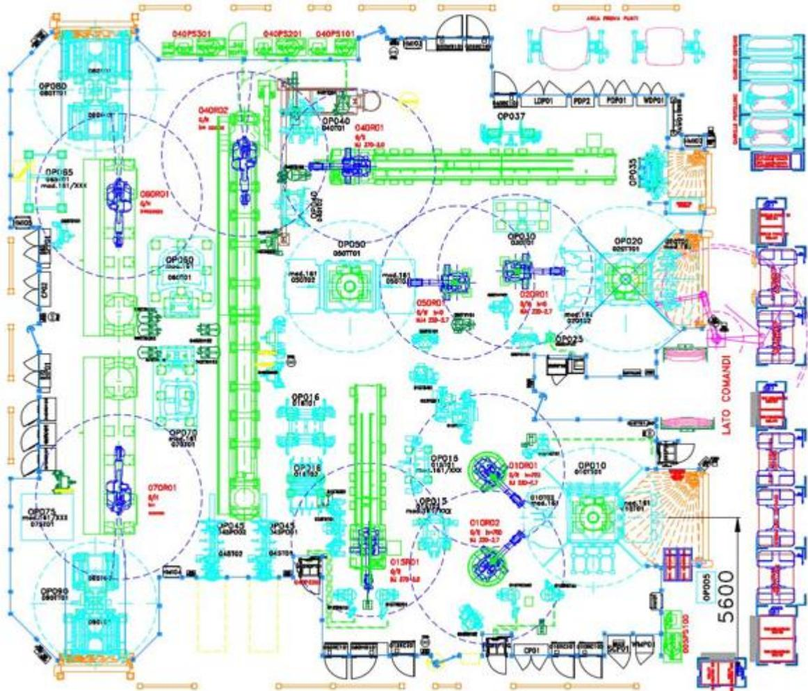
Figure 25 – Hood/ tailgate pre-assembly cells layout, Mirafiori Plant
