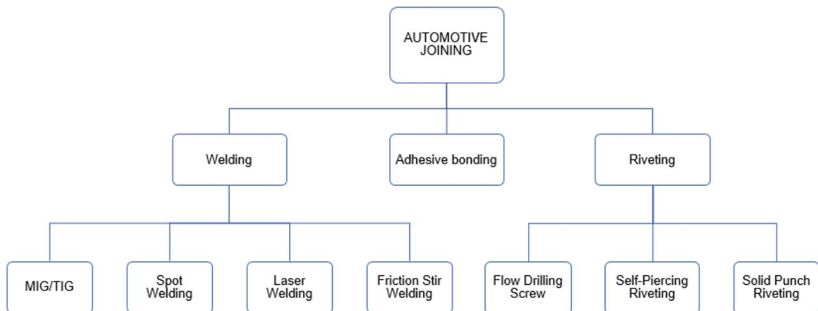
Figure 12 - The most common joining processes in automotive
