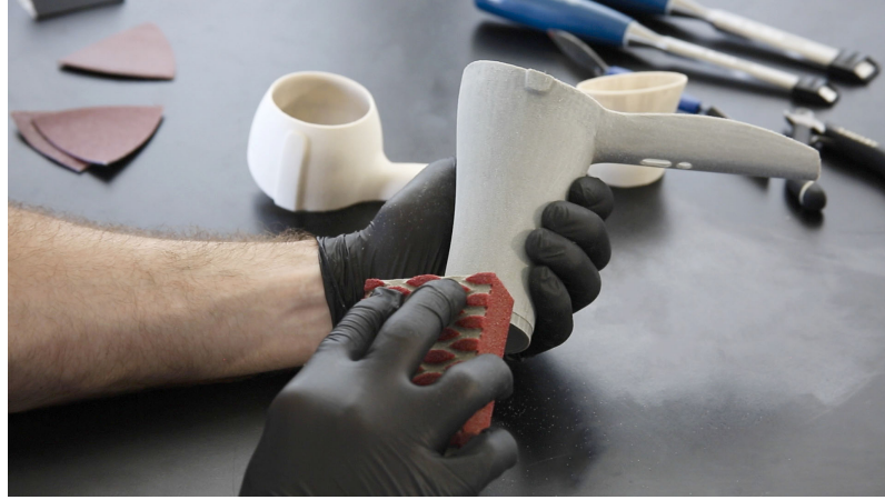
Figure 1.11: Sanding, and example of Post Processing technique [33]
