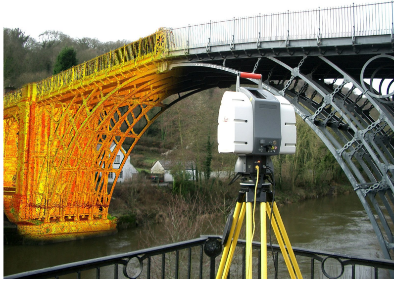
Figure 1.5: 3D laser scanning the geometry of a bridge [11]
