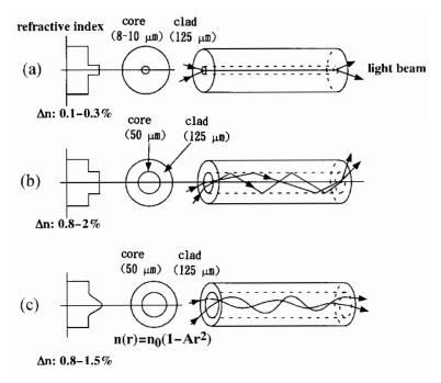
Figura 1.2. (a) Fibra Single-mode, (b) Fibra Multi-mode di tipo step index, (c) Fibra Multi-mode di tipo graded index. [1]
