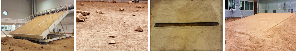
(a) Tilting Platform inclined at 30^\circ . (b) Rocks in the Main Arena. (c) Crevasse of 15 cm depth. (d) Slope of 10^\circ .
