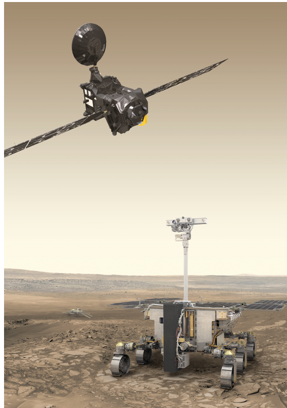
Figure 1.1: ExoMars 2020 Rover in foreground, the Surface Platform in background and the Trace Gas Orbiter on top (Credit: ESA/ATG medialab, EXO-MARS ORBITER AND ROVER, March 27, 2017. From https://m.esa.int/spaceinimages ).
