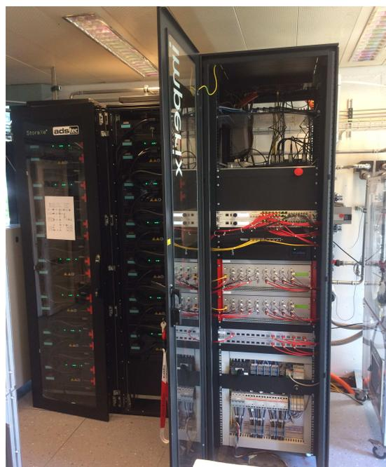
**(b)** In the front there is the converter, directly connected to the battery. The CompactRIO is on the converter box.
