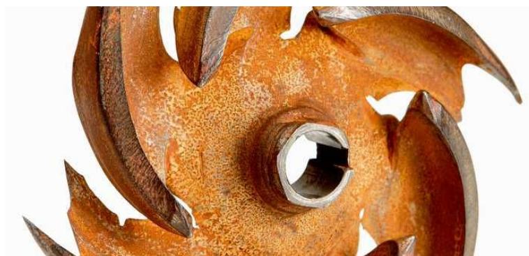
Fig 16 - Centrifugal Pump Cavitation
