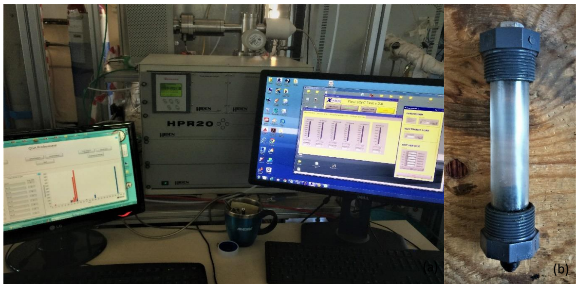
Figure 10: Hiden HPR20QIC mass spectrometer (a) and the reactor for the adsorption tests (b).
