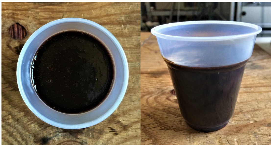
Figure 11: tarry fraction originated from the thermal activation process.
