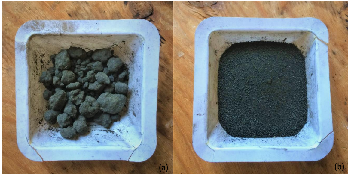
Figure 8: raw and dried sewage sludges as received from the SMAT WWT plant (as received and sieved/milled).
