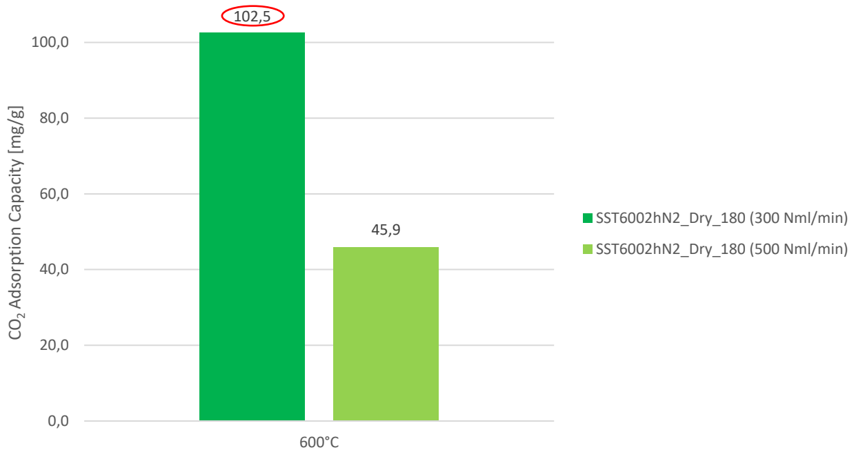
Figure 36: flow rate optimization, comparison between 300 and 500 Nml min -1 .
