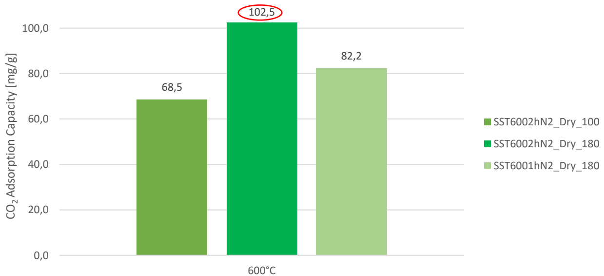
Figure 35: drying temperature optimization, comparison between 100 and 180°C.
