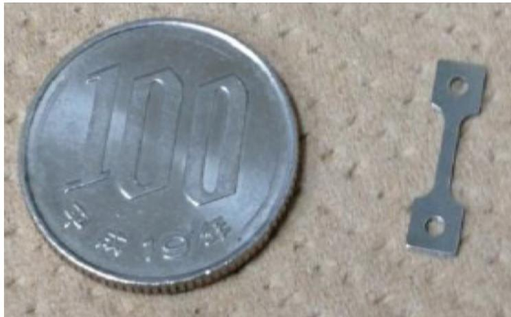
Figure 9: SSJ-type tensile specimen: 16x4x0.25 mm
