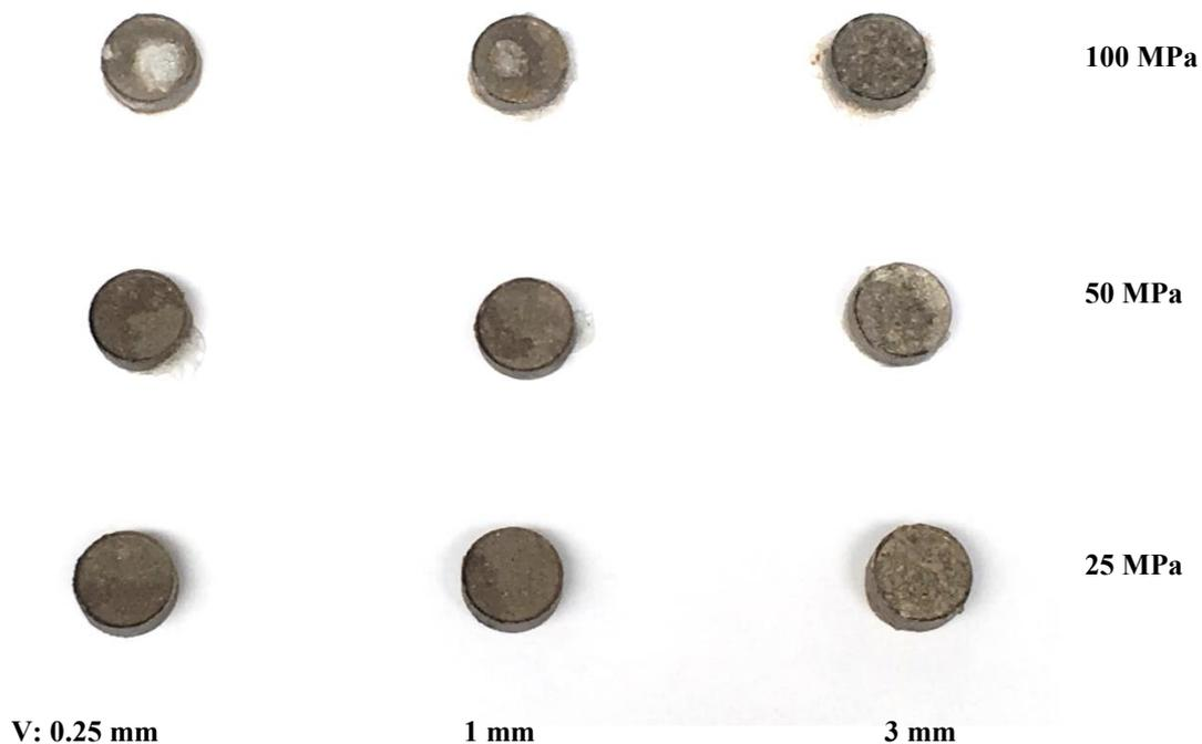
*Figure 36 - Effect of increasing pressures and increasing particle sizes on non-graphitic pure salt pellets.*
