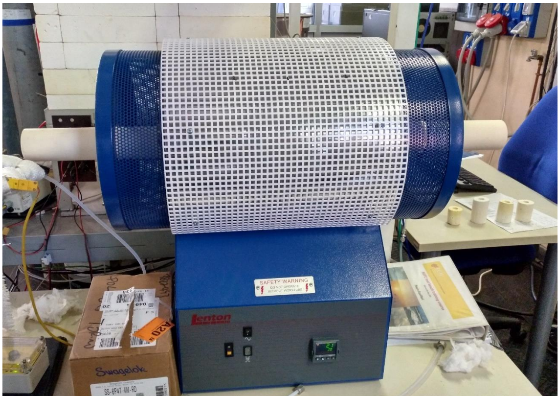
Figure 3.5 The furnace device, on the left side of the picture are shown the alumina cylinders that holds the reactor bar in the work tube.
