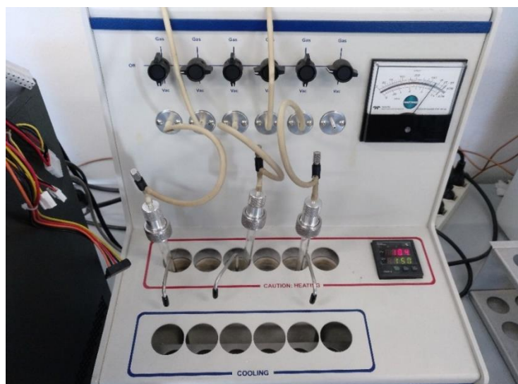
Figure 2.8 Set-up procedure: heat under vacuum to erase organic trace.
