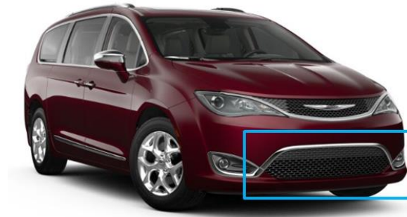
Figure 1-5: AGS is located in the lower grille as shown in the highlighted area [10].
