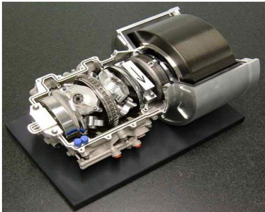
Fig 13. flywheel energy storage used in vehicle xxi
