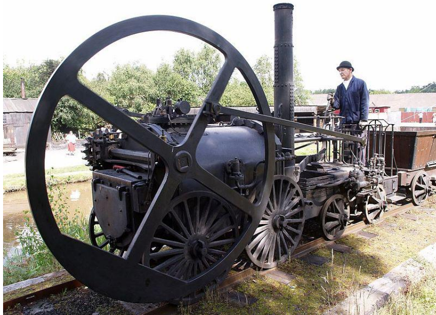
Fig 2. steam locomotive used a flywheel in 1802 ii
