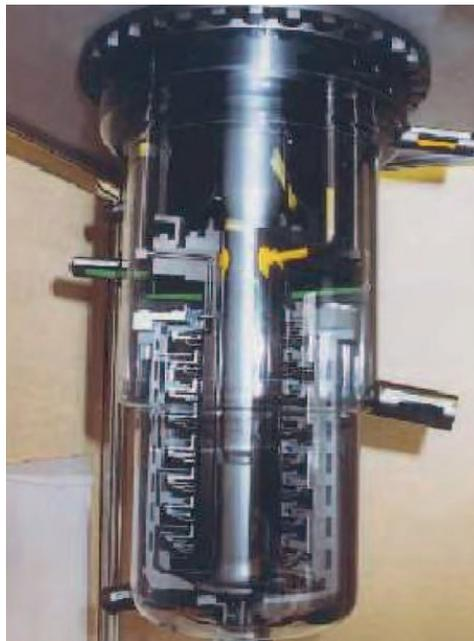
Figure 1.9 - A centrifugal extractor [12]
