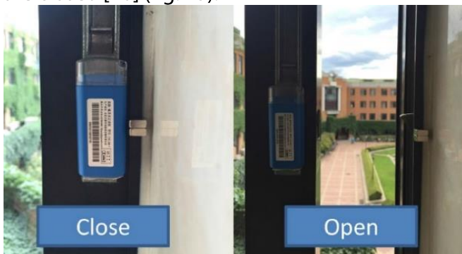
Fig. 15, Features of monitored windows and the magnetic induction device: horizontal sliding window. Source: Shi and Zhao, 2016
