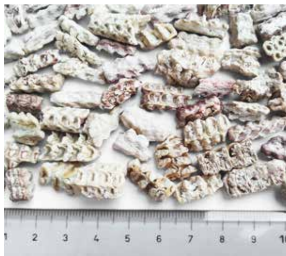
Fig. 6.17 Granulometria Agrindustria 5-10 mm.
