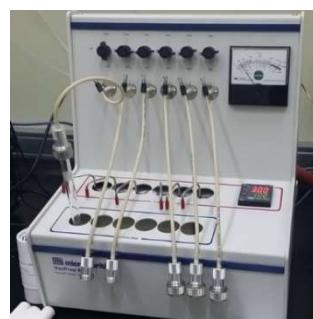
**Figure 2-4:** Furnace for the pretreatment
