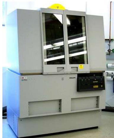
**Figure 2-2:** PANalytical X'Pert Xray diffractometer
