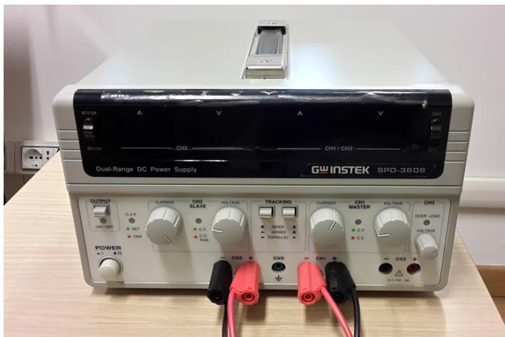
FIGURE 2.8: The power supply SPD 3606 by GW-INSTEK, used to push the motion of the FF at early stages.
