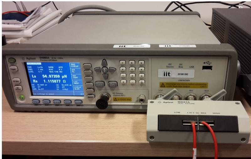
FIGURE 2.22: The Agilent E4980A LRC meter, with band-pass from 20 Hz to 2 MHz, and used to measure the inductive, capacitive and resistive behaviours of the extraction coils; in addition, the Agilent test fixture 16047A is inserted, in order to have a better coupling between coils and instrument.
