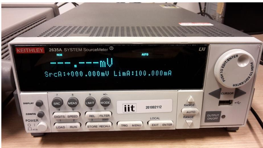
FIGURE 2.23: The Keithley 2635A, a source meter used to measure the intensity of the current induced by EME, and flowing across the extraction coils.
