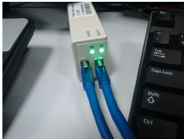
Figure 6.9: Link analyzer when a SpaceWire connection is established
