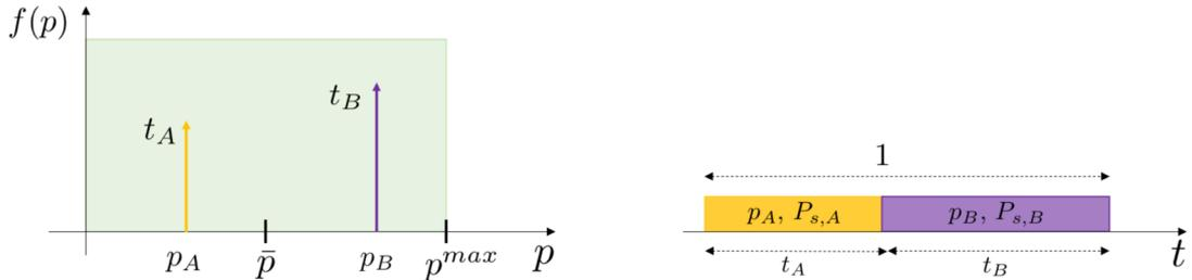
Figure 3.3. Optimal communication strategy. The time frame is divided into two phases (A and B), with the associated parameters:  $p_A$  and  $p_B$  define the relay transmit power of the corresponding phase, while  $t_A$  and  $t_B$  the duration of the phase
