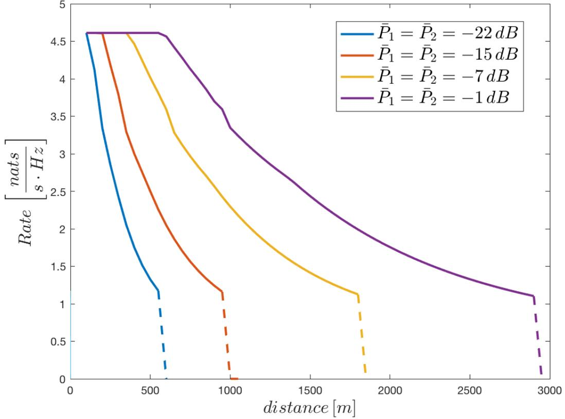
Figure 5.8. Rate values for increasing distance between sources and relay
