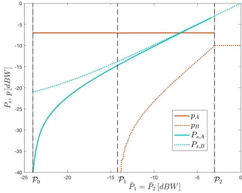
Figure 5.2. Optimal source and relay transmit powers for phase A (solid lines) and phase B (dashed lines)
