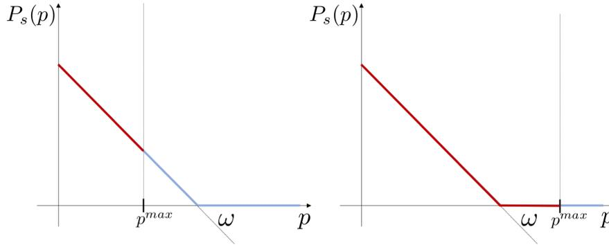
Figure 3.2. Transmission power sum of the sources:  $\omega \geq p^{max}$  (left) and  $\omega < p^{max}$  (right)
