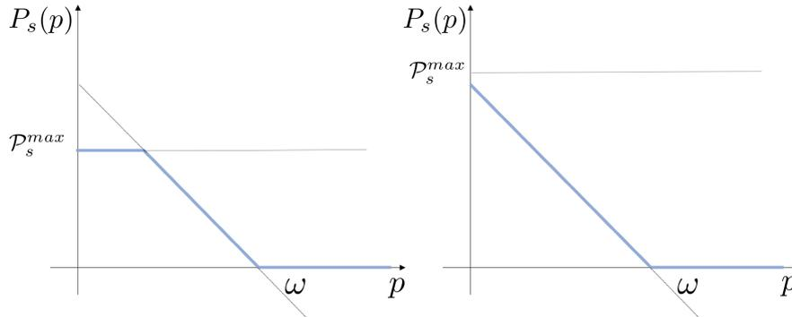
Figure 3.1. Transmission power sum of the sources:  $\omega \geq \mathcal{P}_s^{max}$  (left) and  $\omega < \mathcal{P}_s^{max}$  (right)
